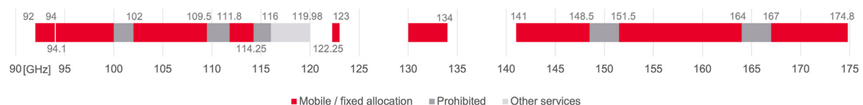
Figure 3. Simplified global allocation mobile / fixed frequency allocation, 92 to 175 GHz
