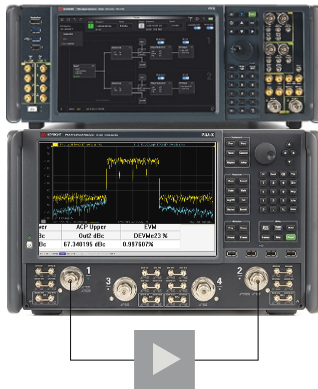
Figure 4. The VCA solution allows the VNA to conduct multiple measurements with a single connection
