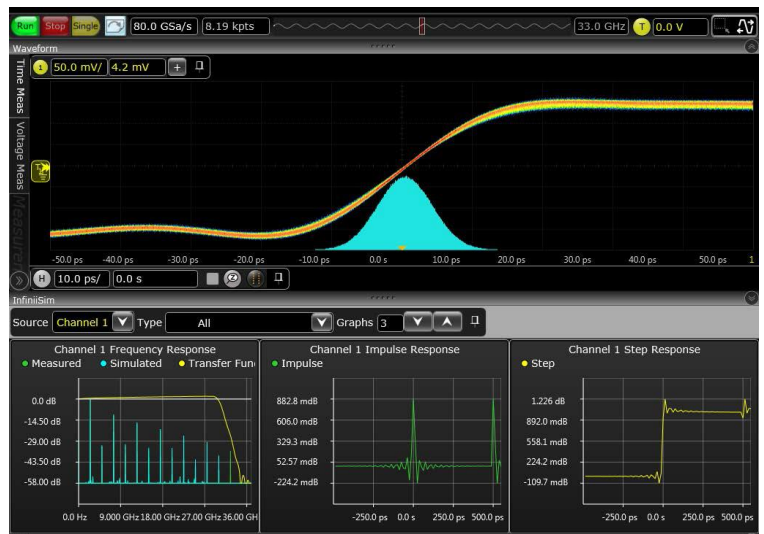
InfiniiSim renders the waveform through hardware acceleration
