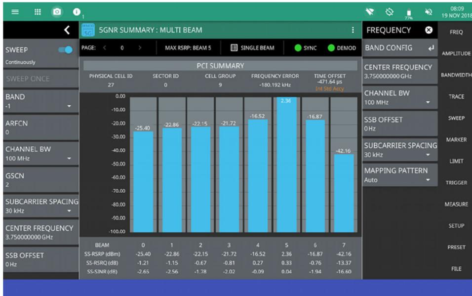
**Figure 6:** Display of 5G beamforming measurement.
