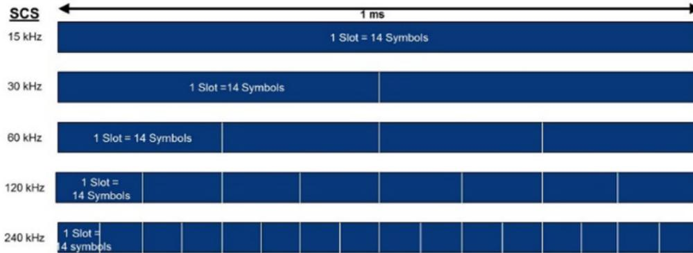
**Figure 4:** Slot structure in 5G.
