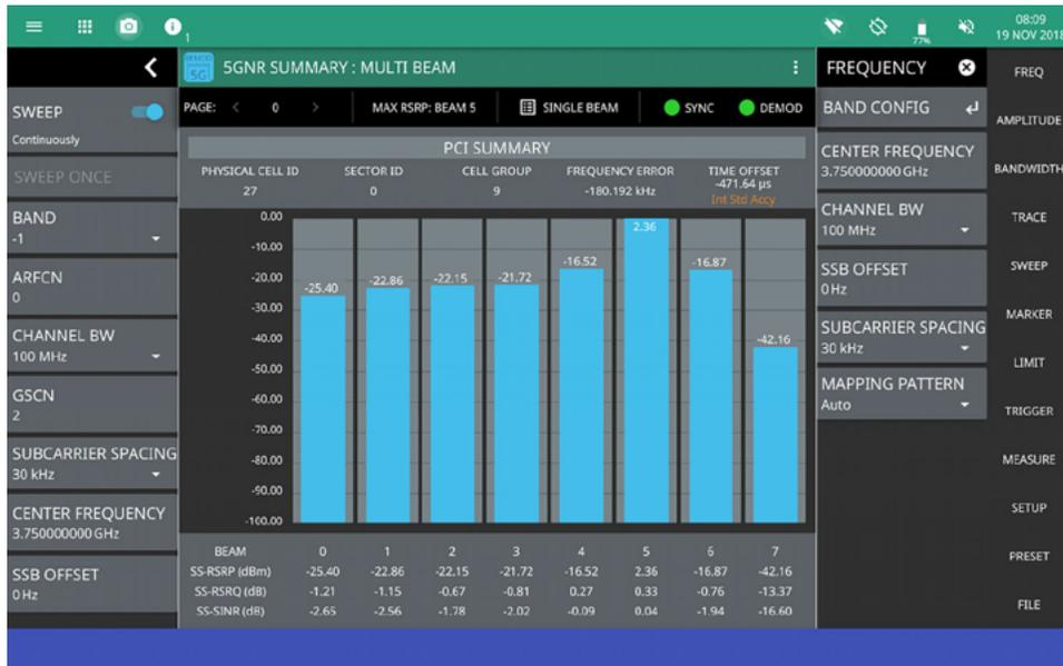
**Figure 6:** Display of 5G beamforming measurement.
