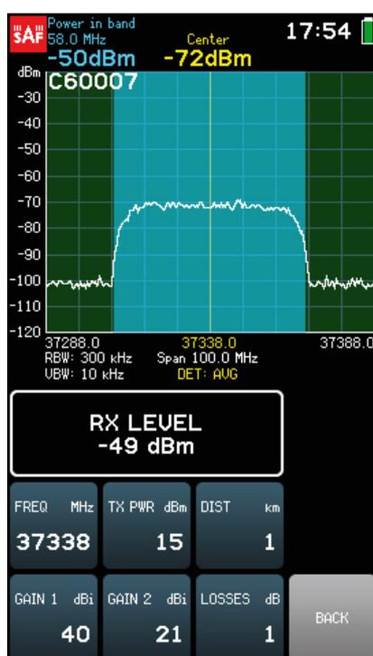
Fig. 2. Typical signal measurement.
