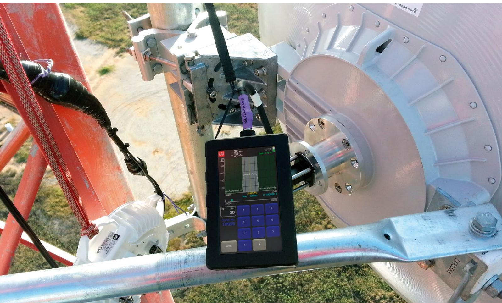
Fig. 3. Spectrum Compact connected to receiving antenna.
