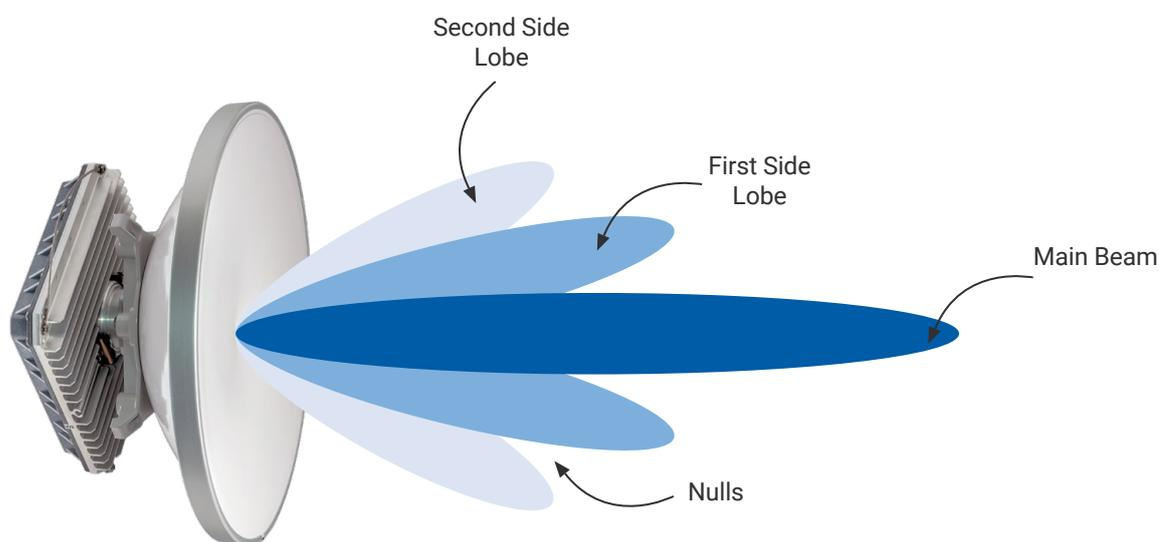
Fig. 6. Side view of the signal propagation
