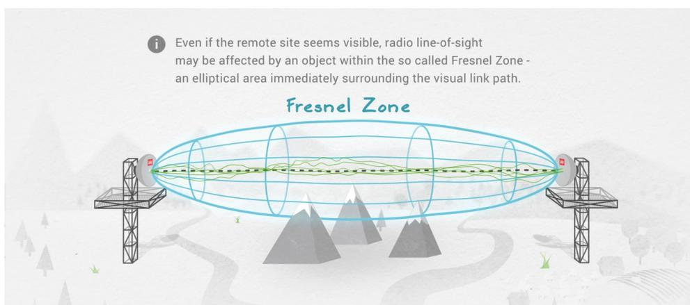
Fig. 5. Geometry of the Fresnel zone.
