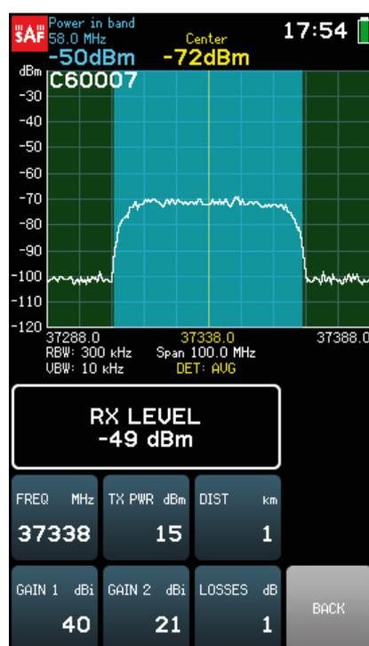
Fig. 2. Typical signal measurement.
