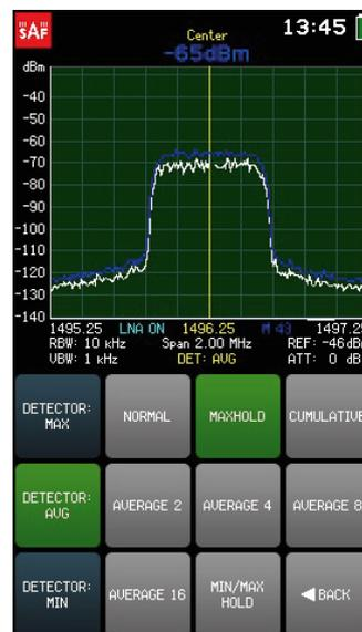
Fig. 10. Example of maximum signal tracing with Spectrum Compact. Blue line depicts maximum achieved through series of measurements.
