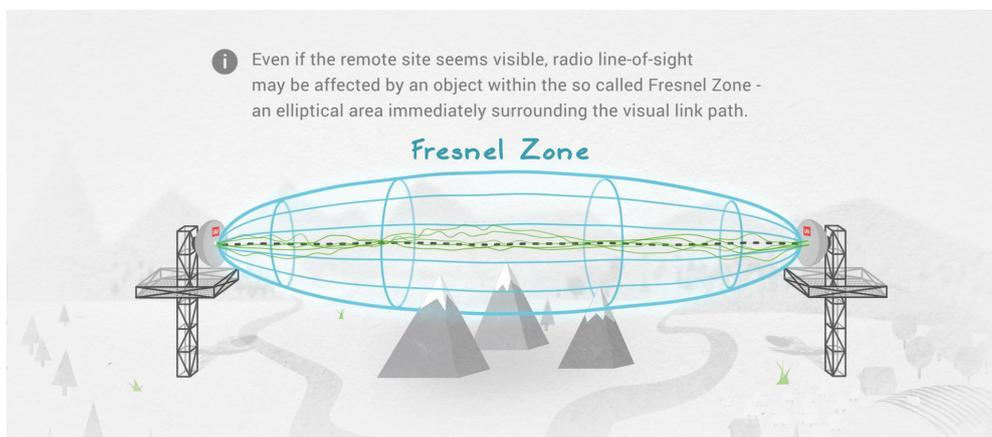
Fig. 5. Geometry of the Fresnel zone.
