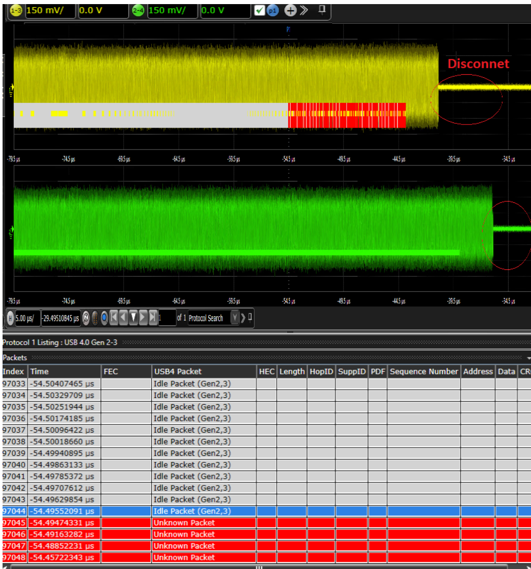
Figure 17. UXR oscilloscope displays inactive Tx and Rx lines
