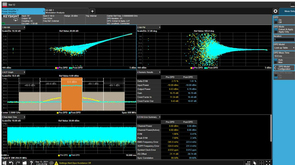
Figure 5. PA after applying DPD
