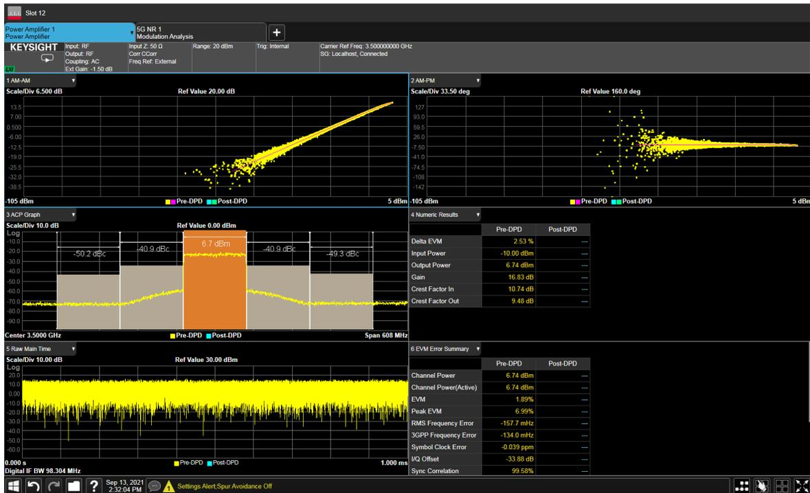
Figure 4. PA before applying DPD
