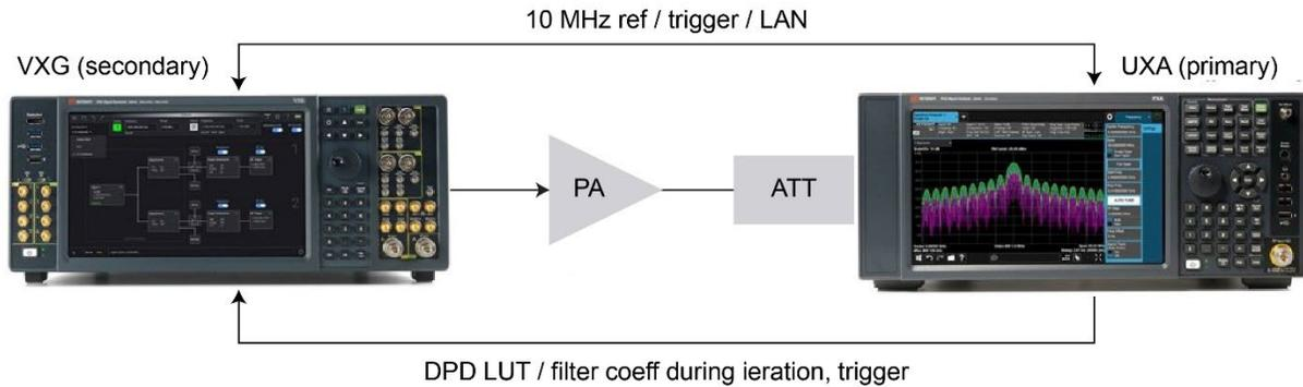
**Figure 3.** Keysight PA and DPD measurement setup
