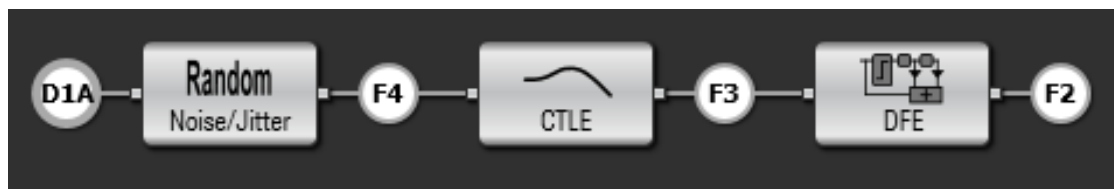
Figure 9. Reference receiver noise and equalizer components
