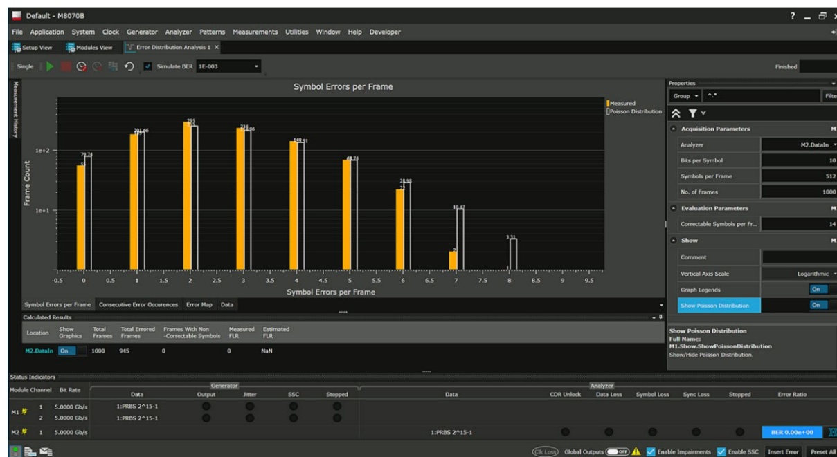
Figure 10. The error distribution analysis M8070EDAB provides multiple views to debug the error distribution. The figure shows an example of symbol errors per frame based on captured pattern streams, with the measured frame loss ratio, based on user-definable number of bits per symbol, correctable symbols per frame and frame length.
