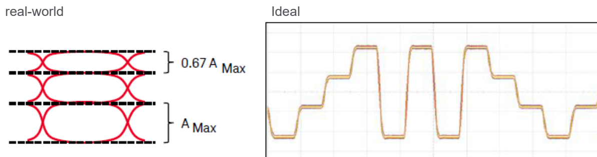
Figure 8. PAM4 eyes can show a level separation mismatch. Receivers must be able to detect the digital signal content properly within the given mismatch ratio.
