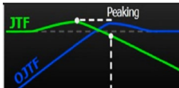
Figure 21. The M8040A provides a built-in- clock recovery option. You can choose between a first and second order PLL characteristic
