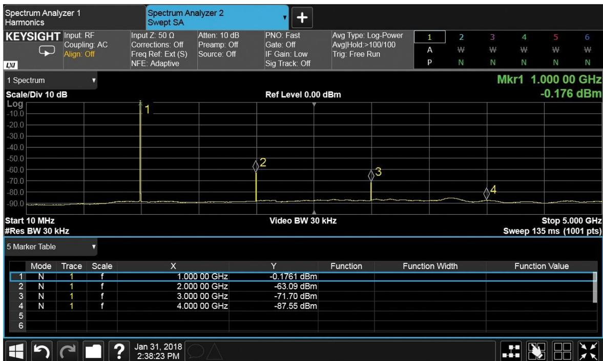
Figure 6. Spectrum analysis with frequency and amplitude readouts
