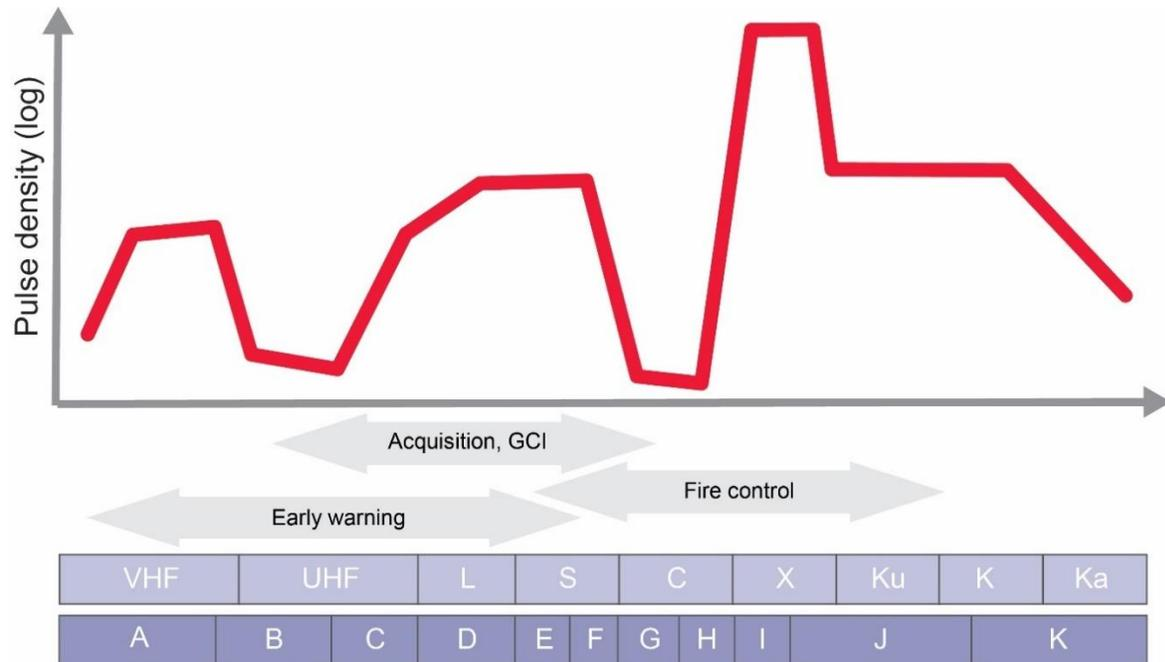
**Figure 11.** A general representation of the threat density vs. frequency band in a typical operational environment. The full RF/microwave environment would combine the threat and commercial wireless environments.
