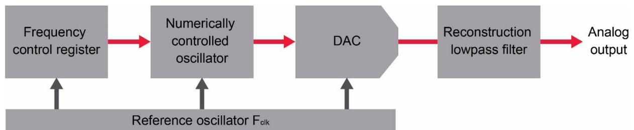
**Figure 15.** Principal functional blocks of a direct digital synthesizer
