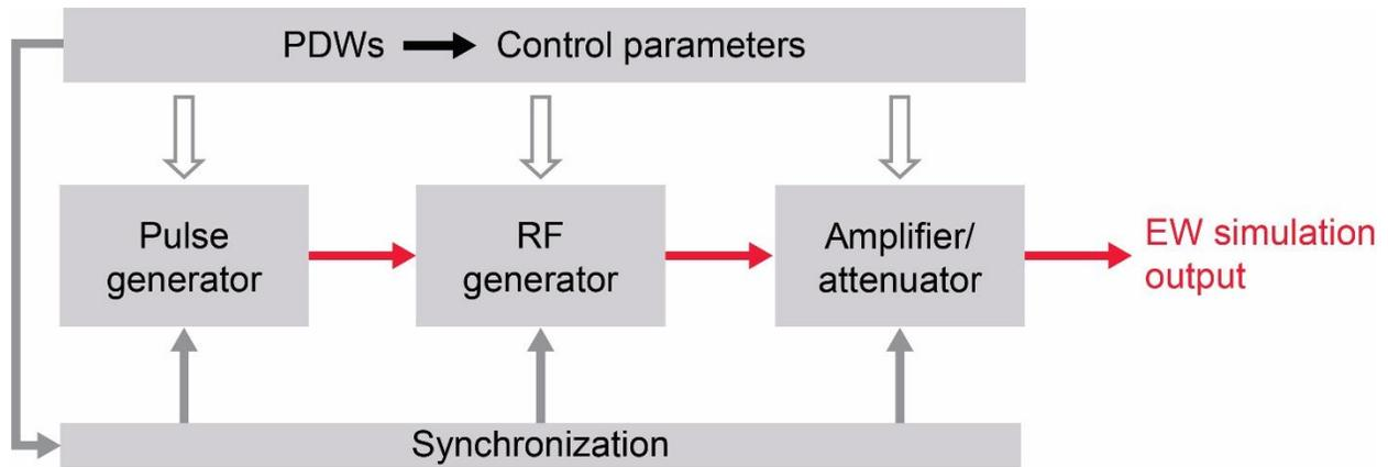
**Figure 13.** In the traditional approach, PDW control parameters are sent in parallel to multiple functional elements, on a pulse-to-pulse basis, to generate and modify the desired signal. This approach results in a complex system, demanding precise synchronization.
