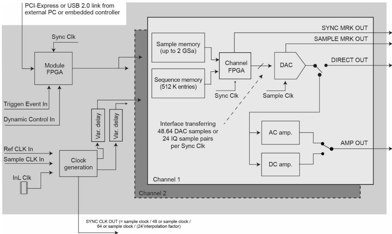
**Figure 9.** Modern Arbitrary Waveform Generators are comprised of much more than DACs. Such new capabilities involve memory sequencing, clock sharing for synchronization, and different output paths to optimize signals depending on the application. Shown here is the block diagram for the high-resolution M8190A Arbitrary Waveform Generator.
