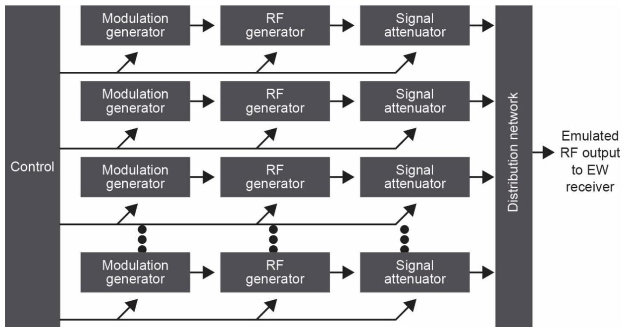
**Figure 14.** A signal generation approach using separate functional elements can be scaled up to increase pulse density and generate a more realistic environment. The cost and space requirements scale up rapidly as well <sup>2</sup>.
