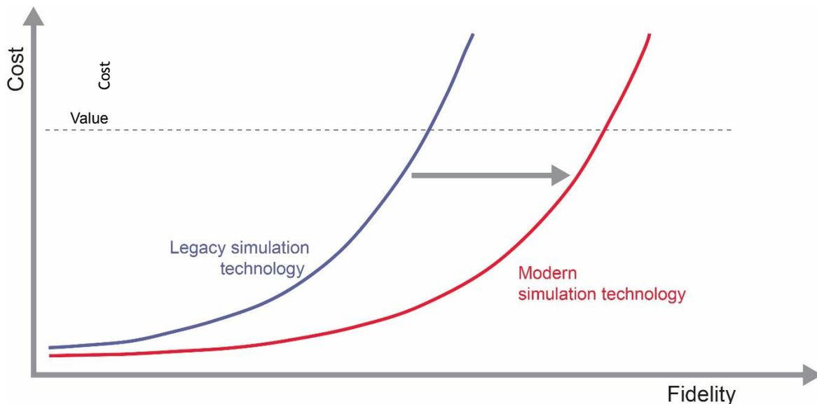
**Figure 12.** Simulation fidelity and cost increase exponentially. System integrators and evaluators must determine the level of cost versus fidelity to ensure system performance. New simulation technologies enable more simulation realism and fidelity at a lower cost.
