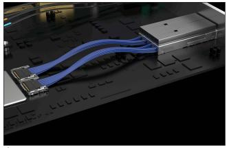
▲ Fig. 3a Image of Samtec's Double Density Flyover QSFP cable system connecting to Si-Fly<sup>®</sup> interconnect.
