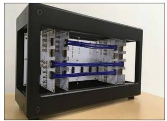
Fig. 2 Samtec's PECFF Emulation Platform showing configurable cabled topologies between mock GPU cards in a typical AI/ML system architecture.
