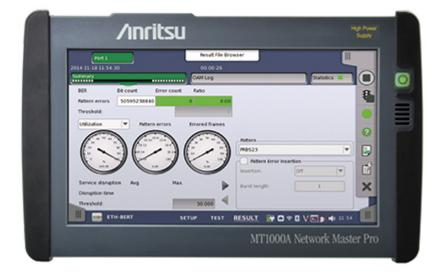
**Vienna, Austria, October 6, 2021** – Anritsu Corporation has added a function for PTP wander, a metrics for evaluating frequency variations as low as 10 Hz to the PTP\*1 network time synchronization error to the company's smallest-in-class 100 Gbps Network Master Pro MT1000A.
