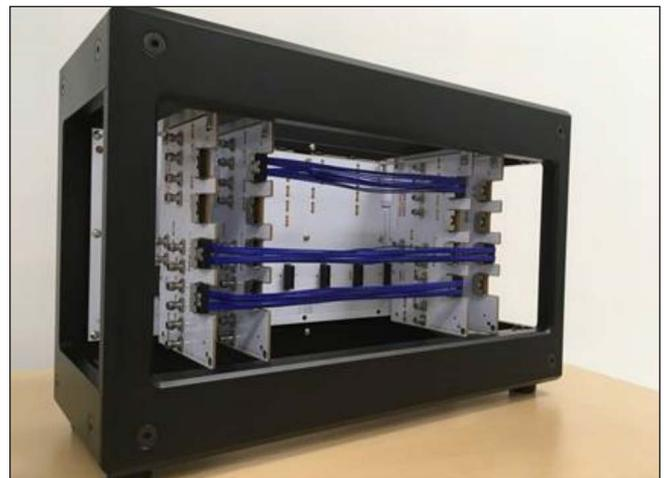
▲ **Fig. 2** Samtec's PECFF Emulation Platform showing configurable cabled topologies between mock GPU cards in a typical AI/ML system architecture.
