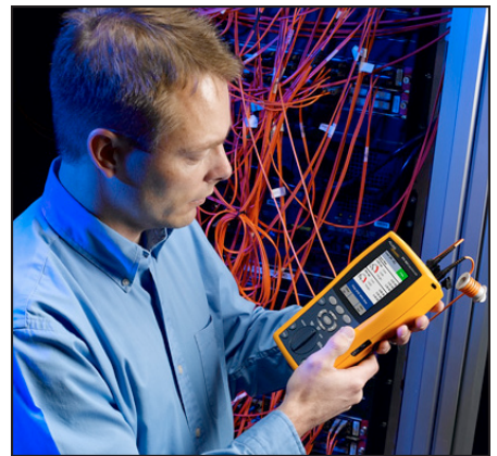
The Fluke Networks DTX CableAnalyzer with Fiber Modules provides a reliable method for loss-length certification.
