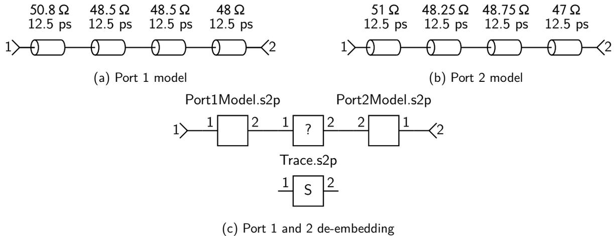
Figure 5: Impedance peeling de-embedding
