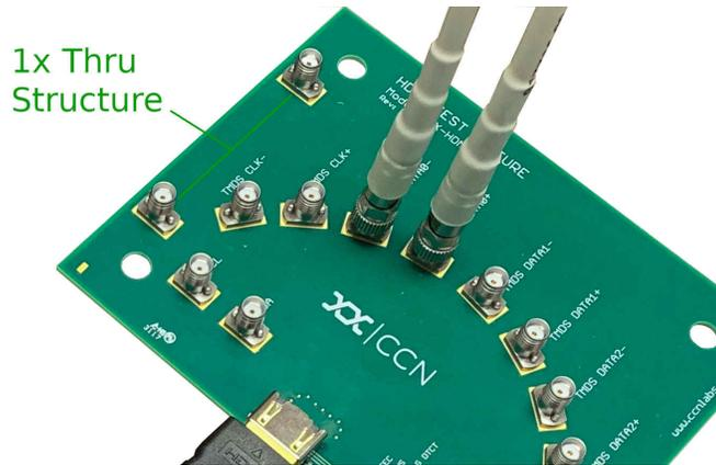
Figure 3: Fixture with 1× thru de-embedding structure (used with permission from CCN, [www.ccn1abs.com](http://www.ccn1abs.com))
