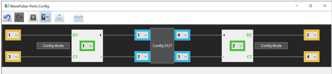
Figure 11: WavePulser 40iX mixed-mode conversion setup
