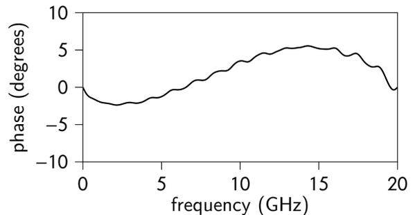
(f) Phase (with 442.74 ps delay removed)
