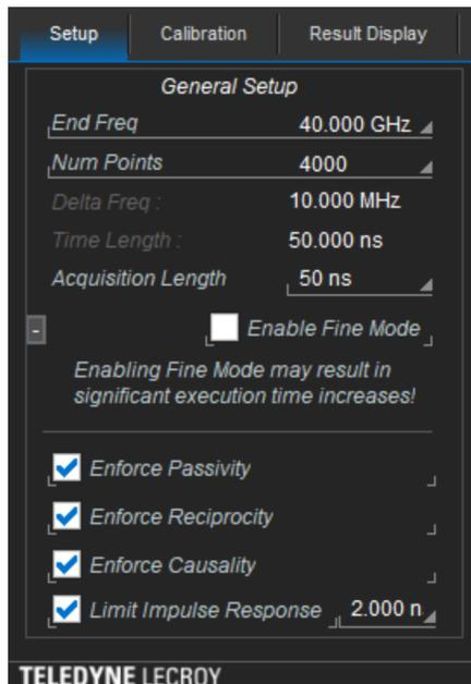
Figure 6: WavePulser 40iX setup
