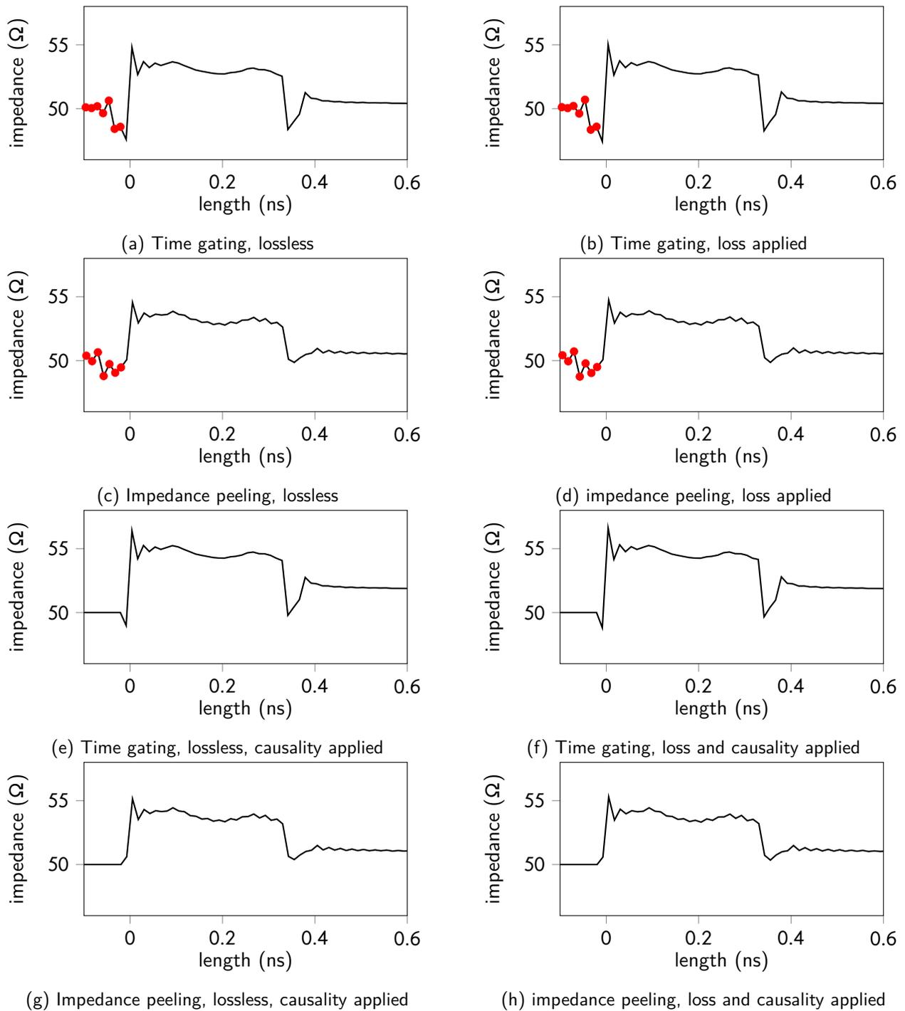
Figure 9: Resulting impedance profiles under various peeling and gating conditions
