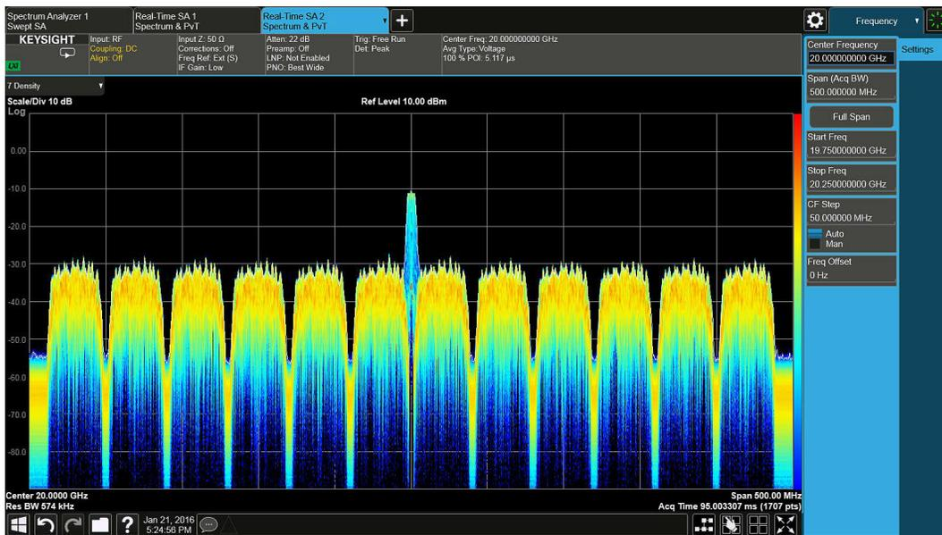
**Figure 21.** RTSA for interference detection.
