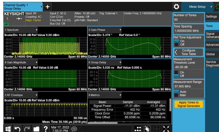
**Figure 9.** Example group delay measurement example using wideband filter as DUT. Top right shows phase trace, middle left magnitude trace, middle right group delay trace, bottom left RF envelope trace, and bottom right displays assorted metrics.
