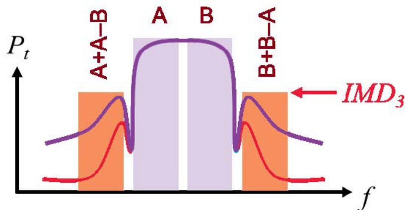
Figure 12. Non-linear distortion in PA creates interference in adjacent channels.
