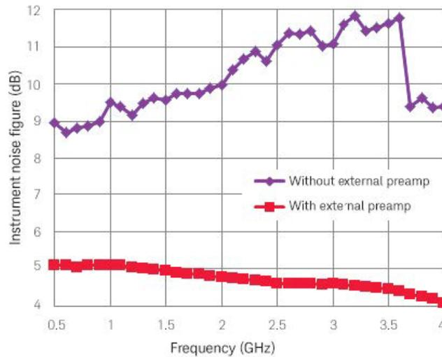
**Figure 4.** Effective instrument noise figure without external preamp (purple line, diamonds) and with external preamp (red line, squares).
