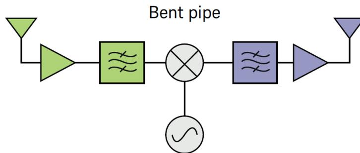
**Figure 1.** Traditional “bent pipe” satellite transponder architecture
