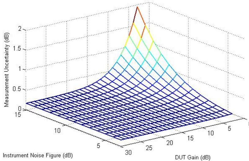
**Figure 3.** Measurement uncertainty results versus instrument noise figure and DUT gain.
