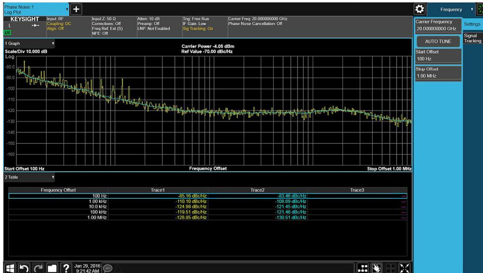
Figure 11. Phase noise measurement example.
