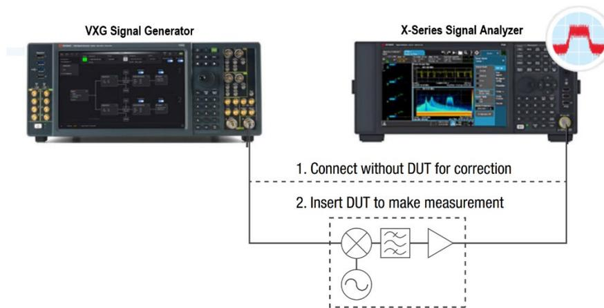
**Figure 8.** VXG signal generator and X-series signal analyzer group delay measurement setup, two steps.
