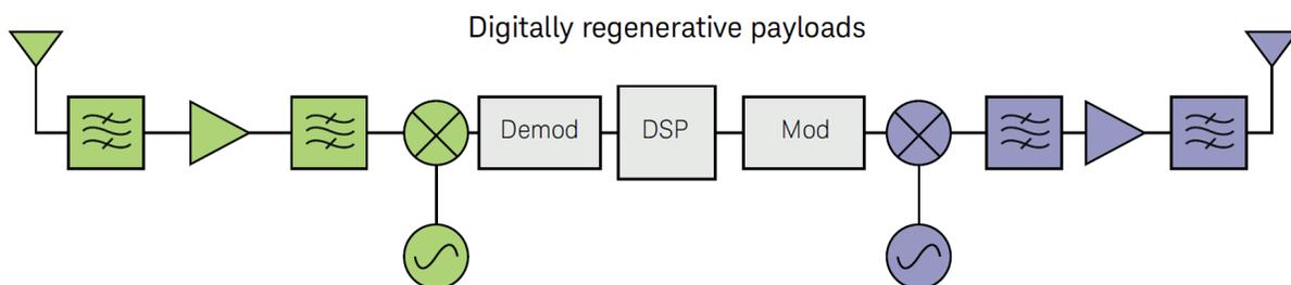
**Figure 2.** Modern “digitally regenerative payload” satellite transponder architecture
