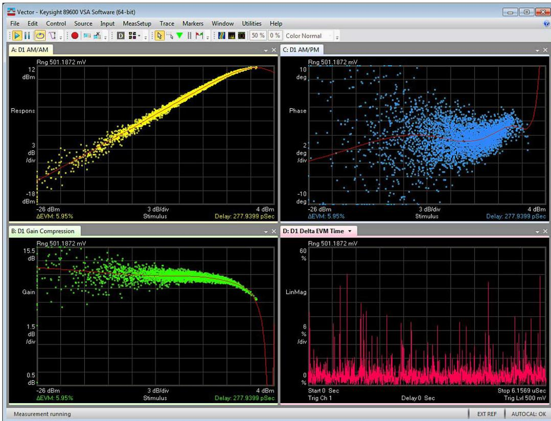
Figure 15. Examples for satellite PA measurements.
