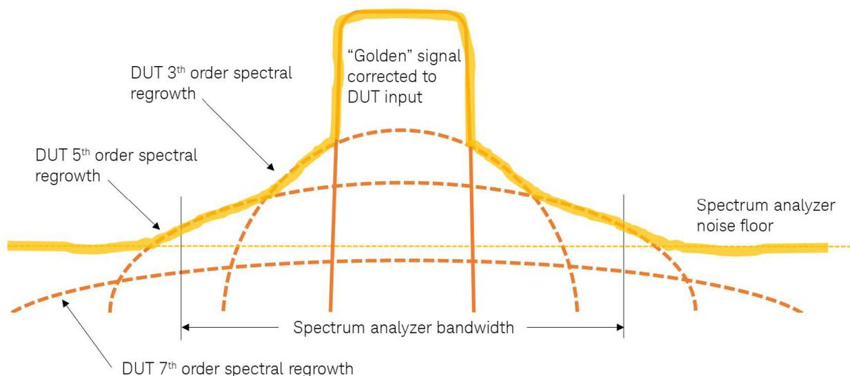
**Figure 14.** Power spread for PA non-linearity effects.
