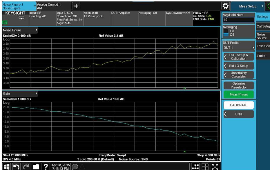
Figure 5. Noise figure measurement on LNA.
