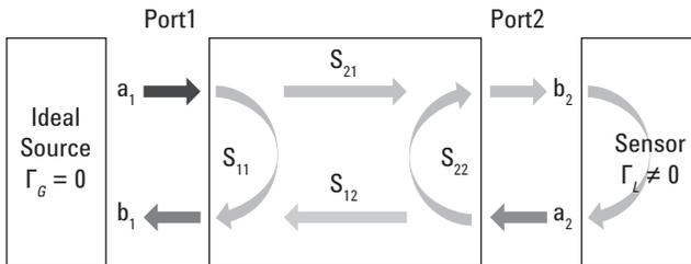
Figure 7. S-parameter correction
