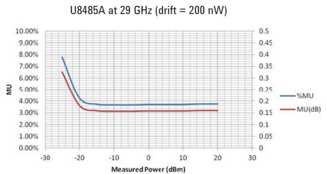
Figure 3. Long term drift performance of U8480 Series USB thermocouple power sensors and its impact to measurement uncertainty over power range
