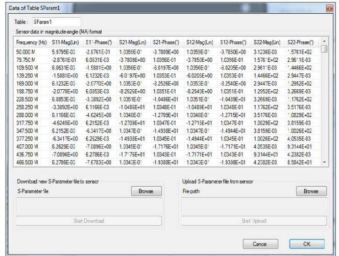
Figure 8. Keysight N1918A power analysis manager enables easy input of the DUT gamma and S-parameter files into the sensor’s memory for gamma and S-parameter corrections
