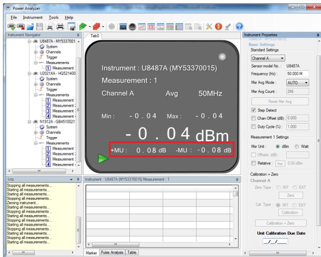
Figure 9. Real-time measurement uncertainty display of the Keysight U8480 Series thermocouple power sensor
