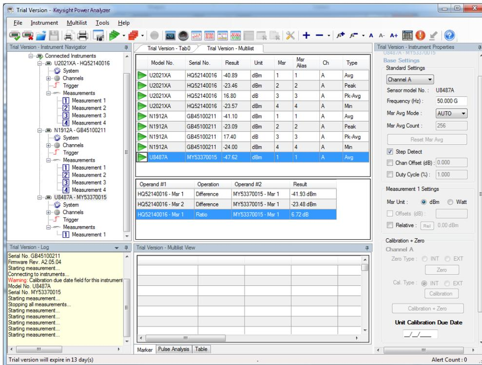
Figure 5. Multi-list display format of Keysight N1918A power analysis manager supports more than 20 USB power sensors simultaneously
