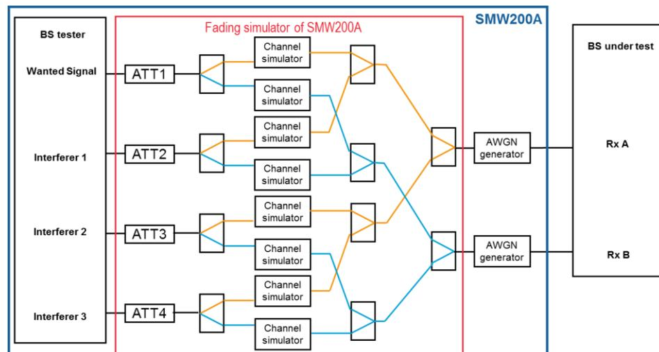
The instrument settings can conveniently be done by selecting the base station test case "8.3.3 ACK missed detection for multi user PUCCH format 1a" in the LTE test case wizard of the SMW.
