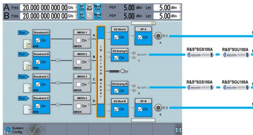
System configuration settings: 4 x 1 x 1 separate sources
