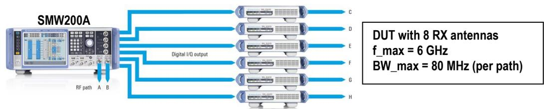
10 MHz reference coupling between SMW and SGTs required.
