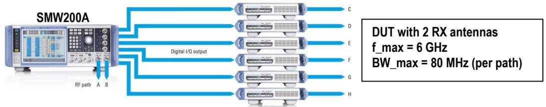
10 MHz reference coupling between SMW and SGTs required.
