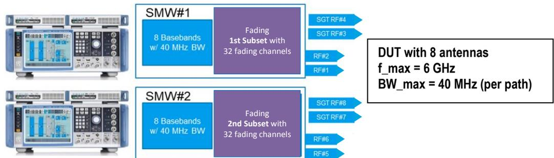
10 MHz reference coupling between the two SMWs and the SGTs is required. A trigger signal is required to synchronize the basebands of the two SMWs. Please see the SMW user manual for a detailed description in section “How to Generate an 8x8 MIMO Signal with Two R&S SMW”.
