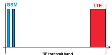
Depending on the supported bandwidth of the DUT, this can mean that a multitude of carriers needs to be generated by a test signal generator.
