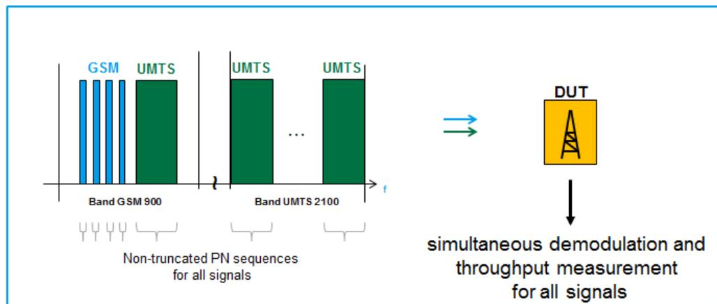
If many of these carriers are to be generated via a single multi-carrier waveform the waveform size is generally getting too big for a signal generator to be played back, especially if the spacing between the carriers is big.
