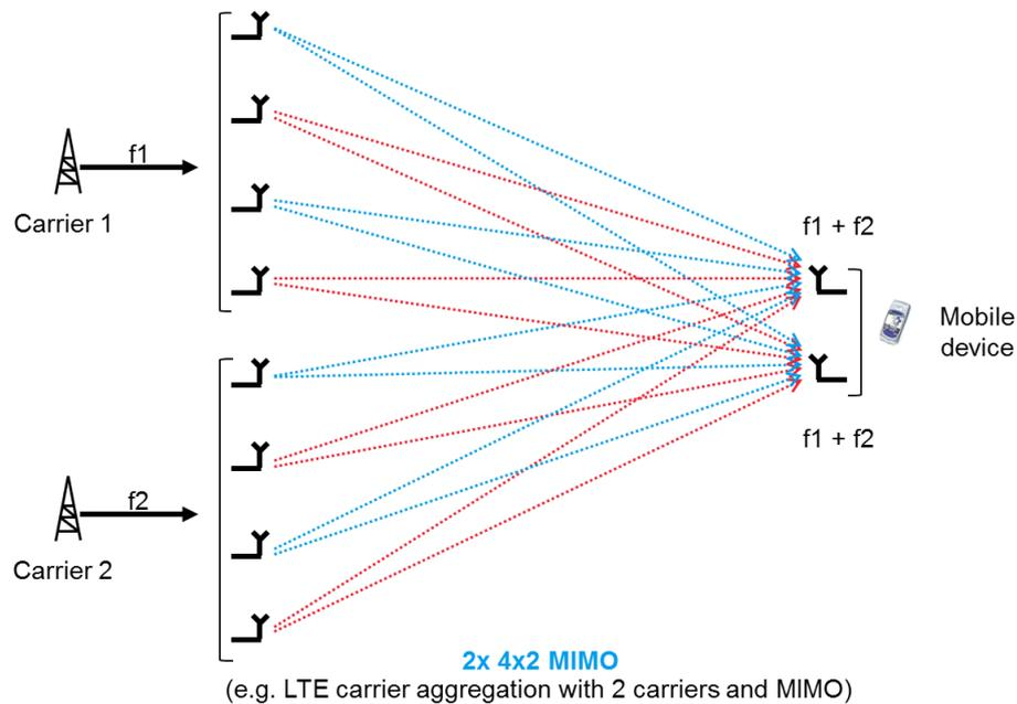
For intra-band carrier aggregation, the number of receive antennas at the DUT determines the number of required RF outputs of the signal generator. For inter-band configurations, the product of “number of receive antennas at the DUT” times “number of inter-band carriers” determines the number of needed separate RF chains.
