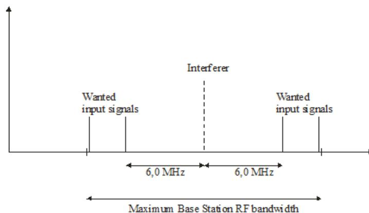
Figure 7.8-1 Allocation of wanted signals and interferer
