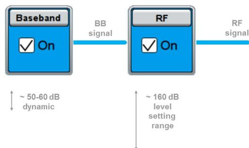
In consequence this means as a rule of thumb that for the generation of multi-channel signals it has to be distinguished whether the needed total dynamic range is more or less than 50 dB. If all signal components fit within 50 dB dynamic range, then adding the signals in the baseband is possible. Otherwise separate RF signal generation paths should be used and the signal components need to be added at RF via RF combiners to meet the dynamic range requirements.
