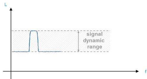
Modern vector signal generators like the SMW have an RF level setting range of more than 160 dB which is achieved via wideband amplifiers in combination with electronic or mechanical attenuators in the RF path. Hence, generation of signals with very high or very low power is easily possible.
