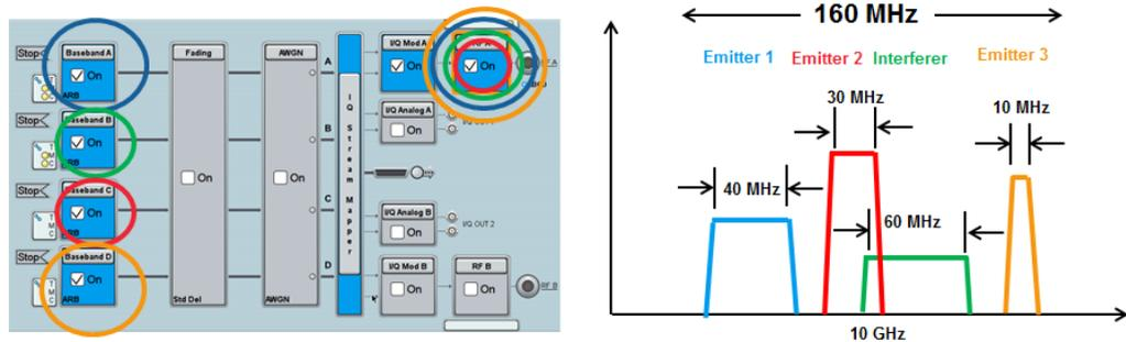
System configuration settings: 4 x 1 x 1 separate sources
