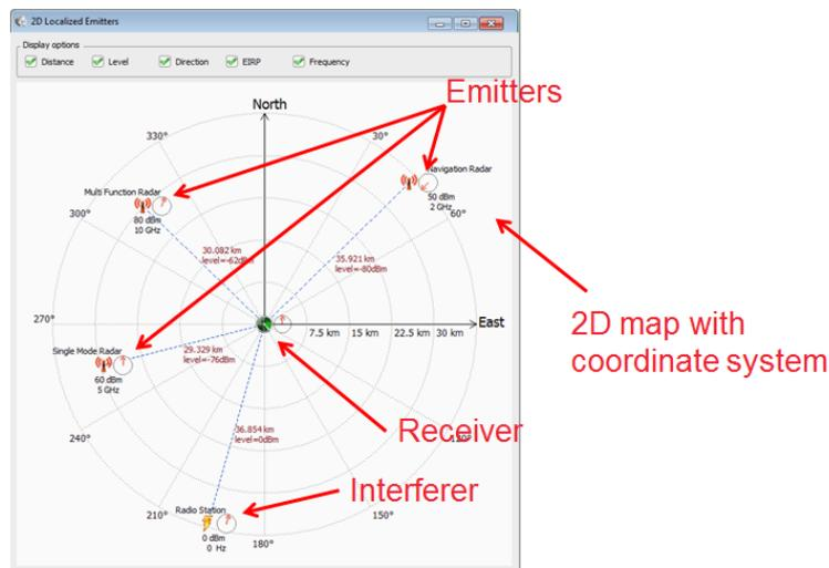
With the SMW-K76 Multiple Entities option up to eight basebands are available in the SMW. Each of these basebands is generally used for generation of one emitter or interferer signal. The individual pulse sequences created by use of the R&S®Pulse Sequencer Software (or the interferers created via WinIQSIM2) are loaded into the ARB generators of the SMW basebands.
