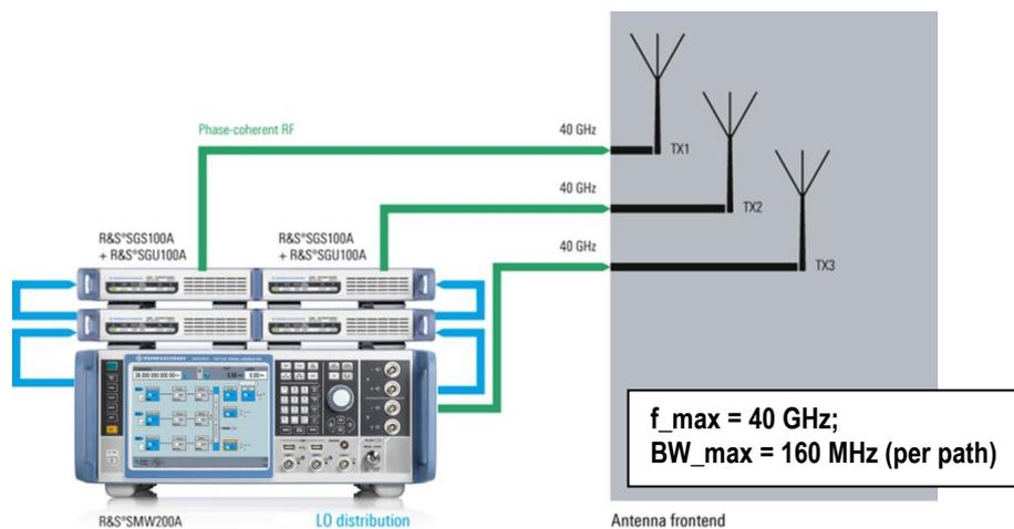
The LO from the SMW is distributed to the two SGS/SGU instruments. It is mandatory to use suitable (phase stable) cables for LO distribution. The baseband signals generated by SMW are distributed to the SGS/SGU via analog I/Q cables.
