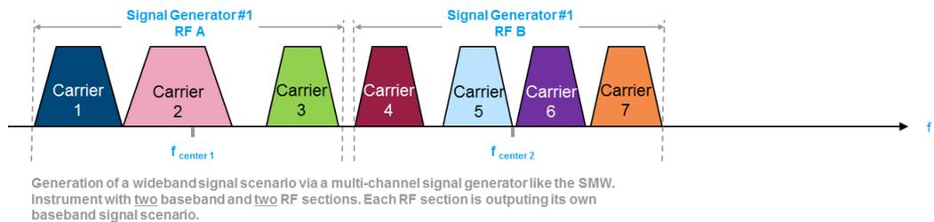
Generally, the higher the number of separate basebands and RF channels that are available in a multi-channel signal generator the more flexibly can such an instrument be used. With a single SMW there is a possibility to have up to eight signal generation paths.
