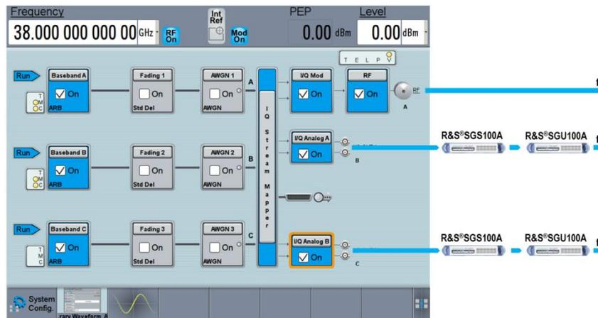
System configuration settings: 3 x 1 x 1 separate sources
