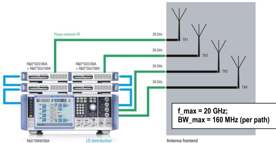
The LO from the SMW is distributed to the two SGS/SGU setups. It is mandatory to use suitable (phase stable) cables for LO distribution. The baseband signals generated by SMW are distributed to the SGS/SGU via analog I/Q cables.
