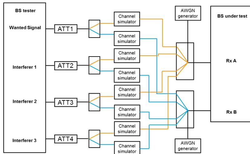
For this test case it is required to generate a wanted LTE signal and three interfering signals. These signals have to be supplied to a DUT with two RX antennas for antenna diversity testing. Additionally, the LTE test signals are faded (ETU70 profile) and AWGN of a certain carrier-to-noise ratio needs to be simulated for every receive antenna.
