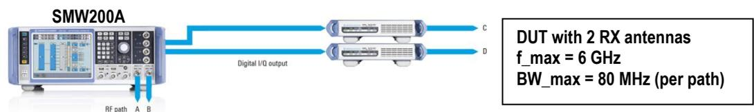
10 MHz reference coupling between SMW and SGTs required.
