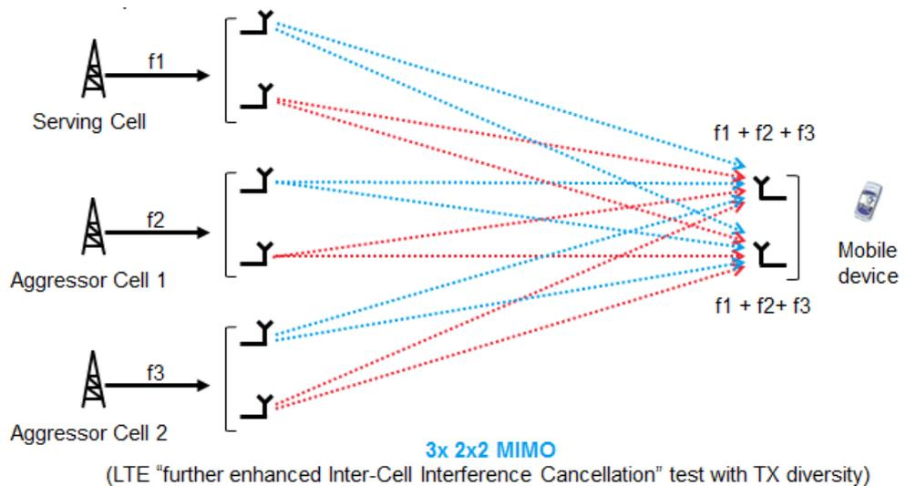
By means of the R&S®SMW200A the required serving cell as well as the two interfering aggressor cells can be simulated by a single instrument
