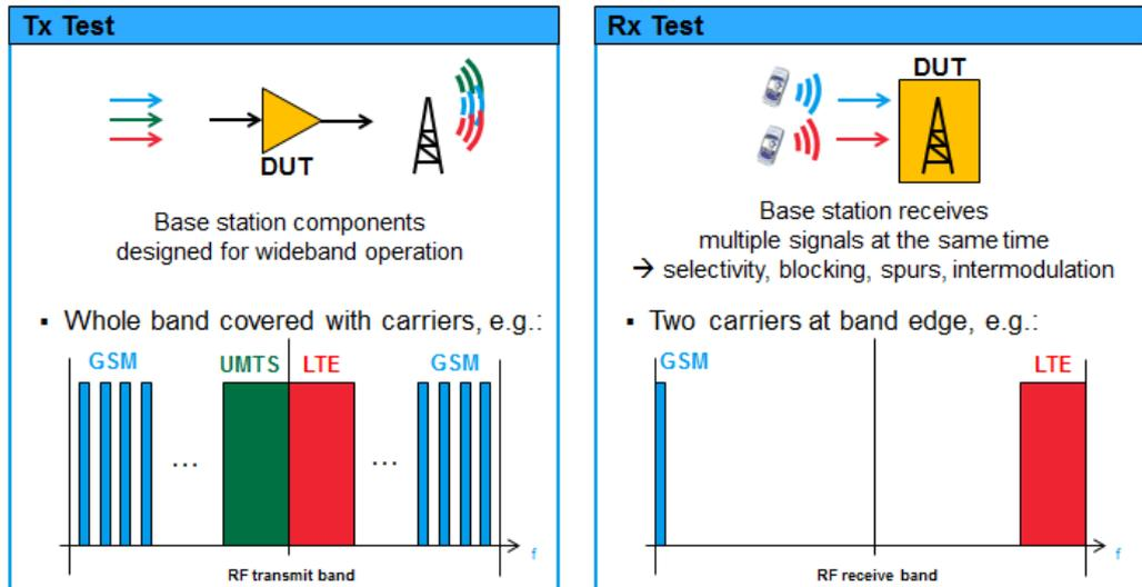
MSR Rx tests require a test signal which consists of maximum two carriers. The carriers can be of same or different radio access technology (RAT) and are typically placed at the band edges. A signal generator is used to generate these test signals to stimulate the receiver.
