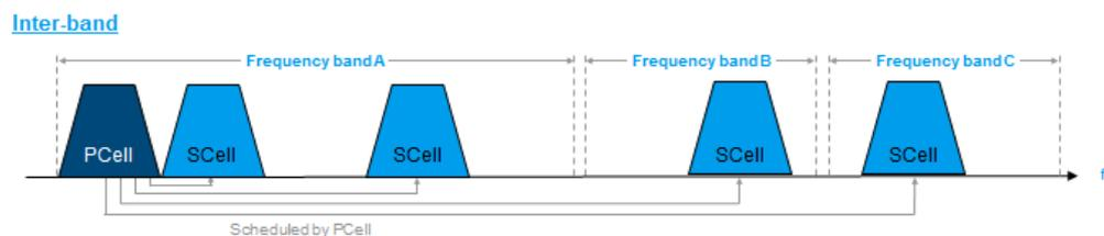
For inter-band scenarios the SMW configuration depends on the spacing between the different component carriers. The SMW features up to two internal RF synthesizers, each with up to 160 MHz bandwidth. I.e. carrier aggregation scenarios with two LTE bands can be covered by a single SMW. More bands can be covered by adding additional SGT vector RF sources to the setup. If required, every component carrier can be placed in a separate frequency band.
