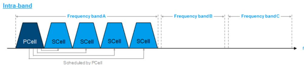
For intra-band scenarios all 5 carriers are added up with frequency offsets/level offsets and output via a common RF path of the SMW.
