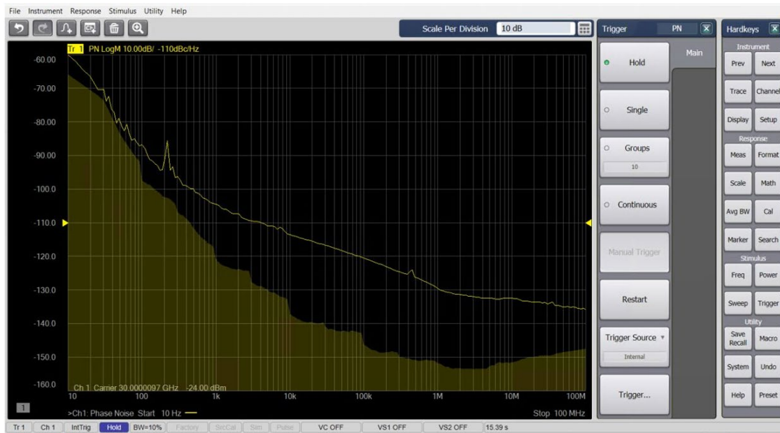
Figure 12. Phase noise measurement with SSA-X
