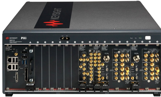
Figure 13. Keysight N5511A Phase Noise Test System (PNTS)
