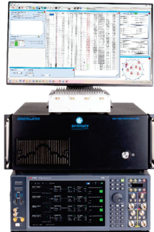
Figure 1. Shown above is an example system including optional 4-channel CRPA receiver (as the DUT)
