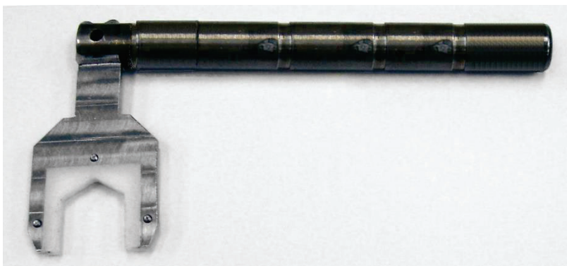
Figure 9. Bent torque wrench
