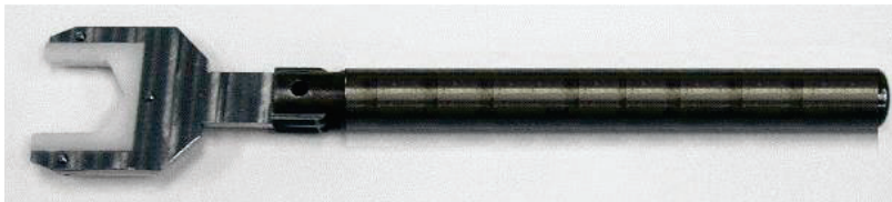
Figure 8. Straightened torque wrench
