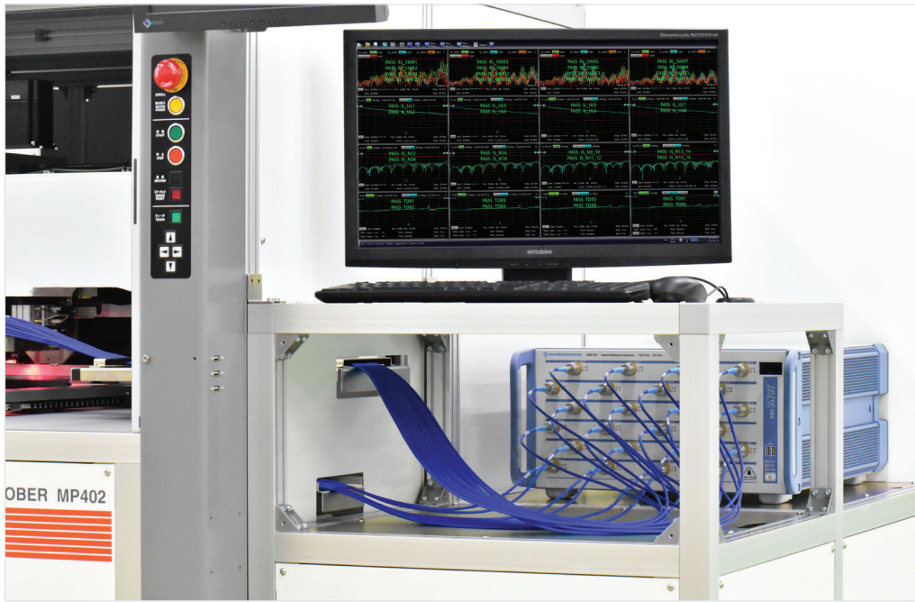
The R&S®ZNB1 is a multiport vector network analyzer offering up to 24 integrated test ports. This VNA platform provides excellent multiport measurements when speed counts.
