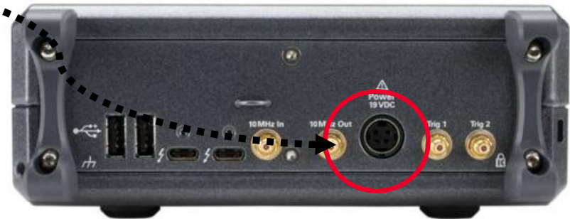
Streamline Series VNA (4- or 6-port model) rear panel
