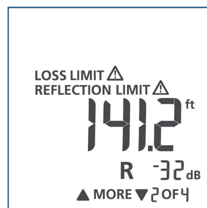
Figure 3. Depiction of a Fiber Troubleshooter showing reflection and loss limits exceeded.
