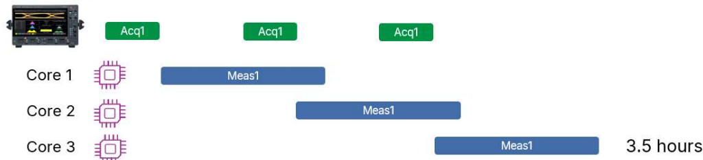
Figure 2. Test times for three different test approaches to make the USB4v2 transmitter feed forward equalization (FFE) measurement. While the multicore oscilloscope is significantly faster than the standard one, this measurement benefits most from server disaggregation.
