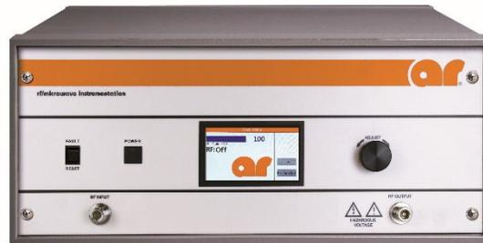
The Model 150W1000B is a solid-state, Class A design, self-contained, air-cooled, broadband power amplifier designed for applications where instantaneous bandwidth, high gain and linearity are required. It will provide a minimum of 130 W across its operating bandwidth. Protection from input overdrive beyond 0 dBm is provided as well as protection from various failure conditions including over-temperature and power supply faults.
