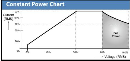
Note: Constant power mode provides increased current at reduced voltage. Maximum available current shown.
