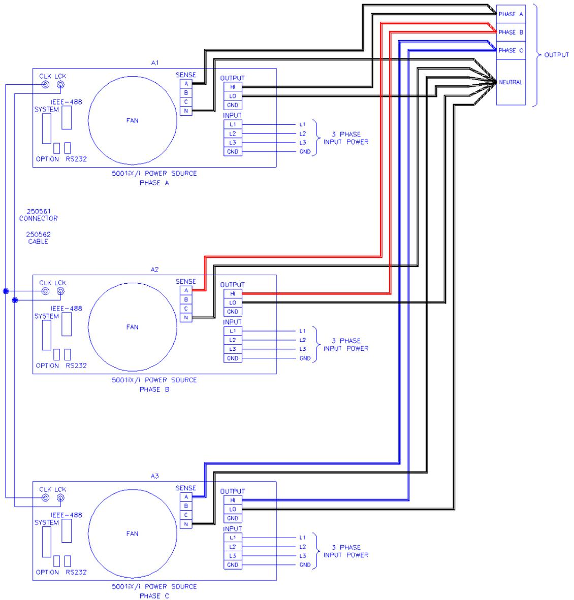
Figure 3-11: Single Phase 15000 VA System (15001X/i)
