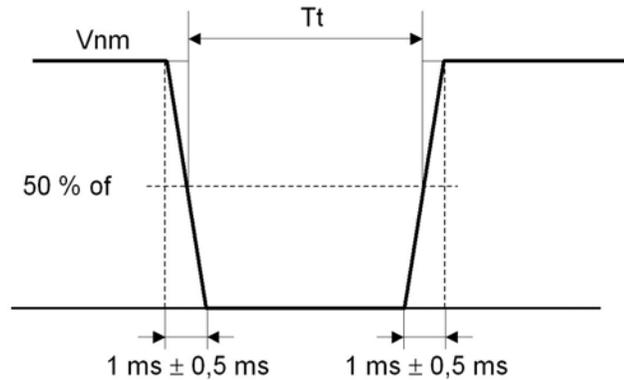
Switching Transients conform Figure B. The T1, T2 and T3 values are shown on screen in the table above the graph. Each permutation shown is repeated one time with a 1 second delay (default) between transients.
