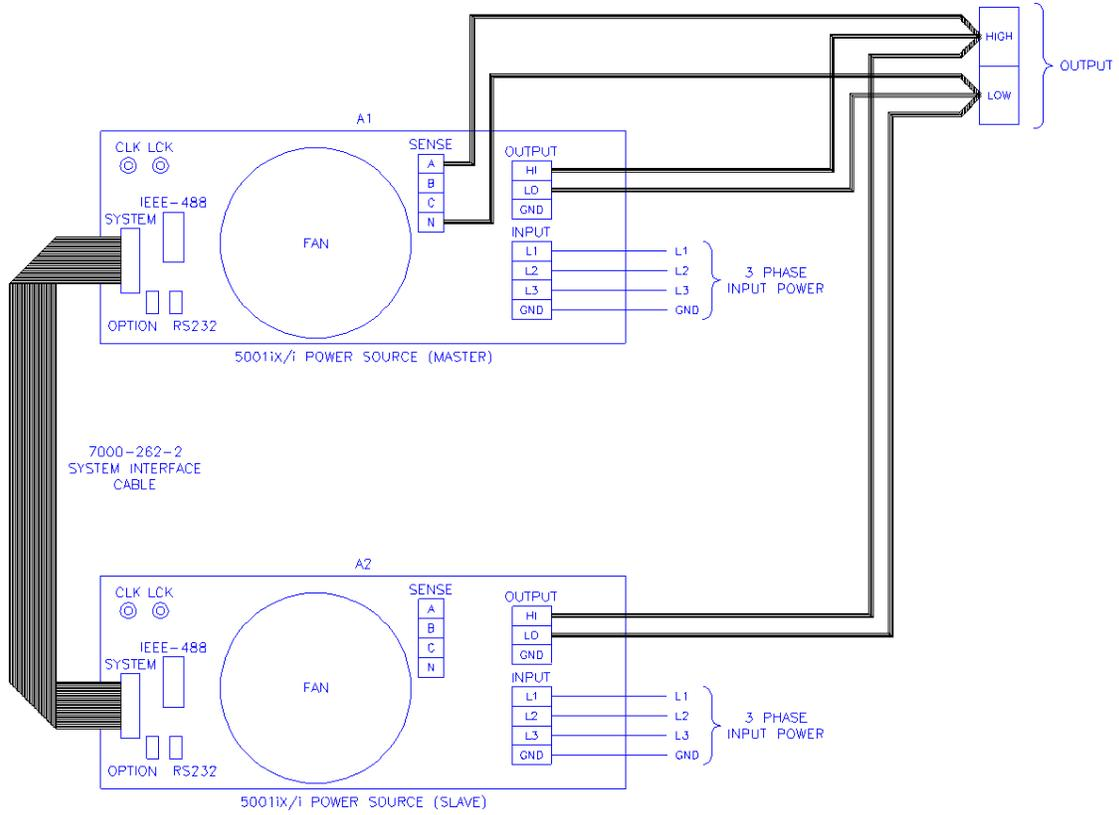
Figure 3-10: Three Phase 15000 VA System (15003iX/i-LK Three Controllers)
