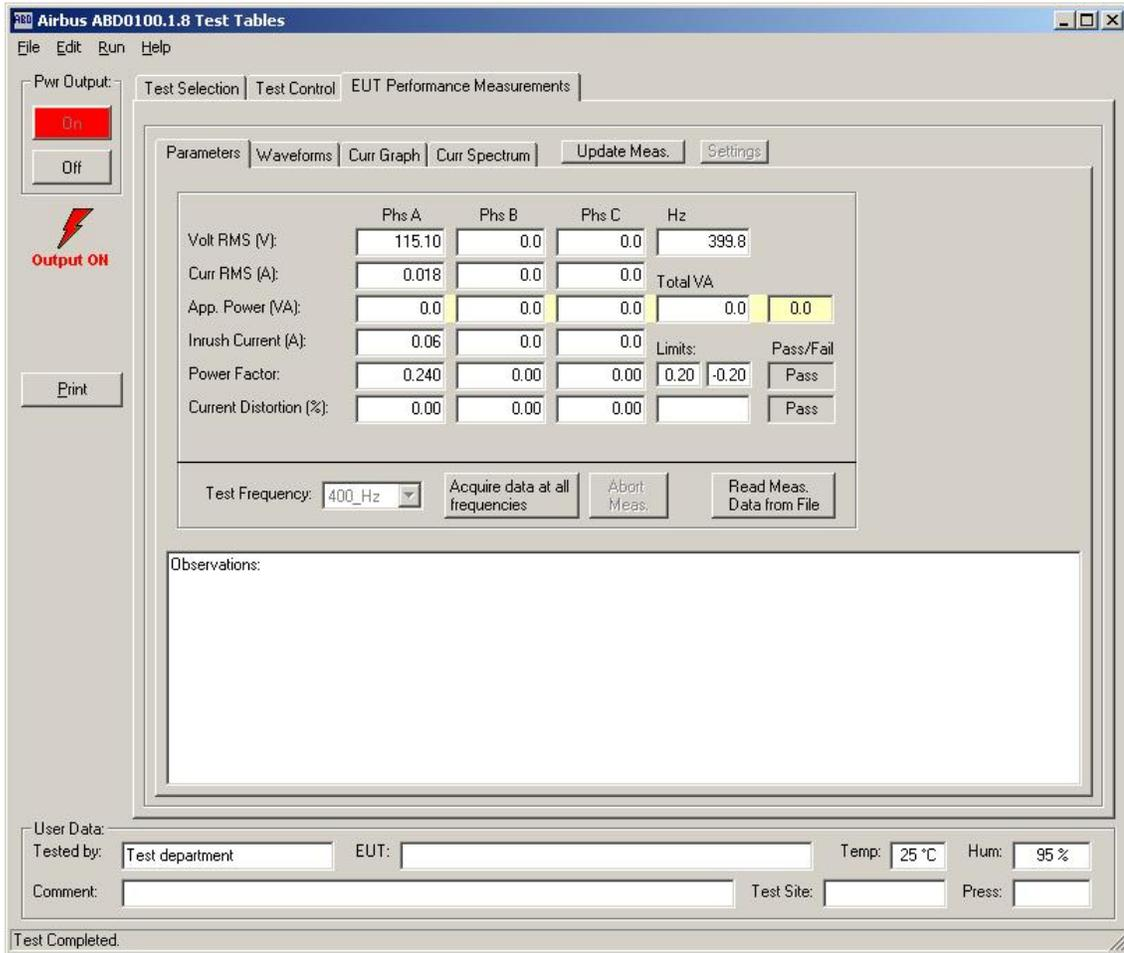
Figure 9-68: ABD Option EUT Measurement Data Screen.
