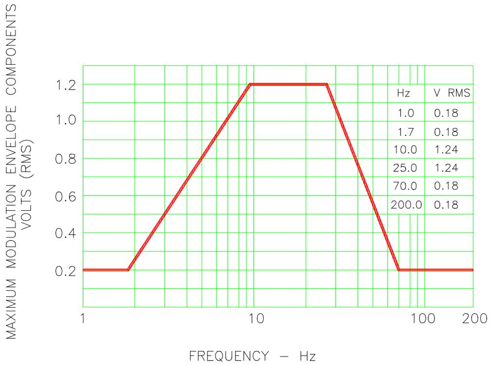
FREQUENCY CHARACTERISTICS OF AC VOLTAGE MODULATION ENVELOPE
