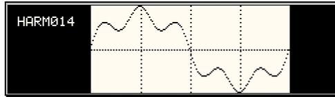
**VIEW(F):** This mode can be used to display any of the available user defined waveforms in a frequency domain display. Waveform data is shown by harmonic amplitude and phase relative to the fundamental frequency. Previewing a waveform can be useful if you are unsure about the nature of the waveform that was stored.
