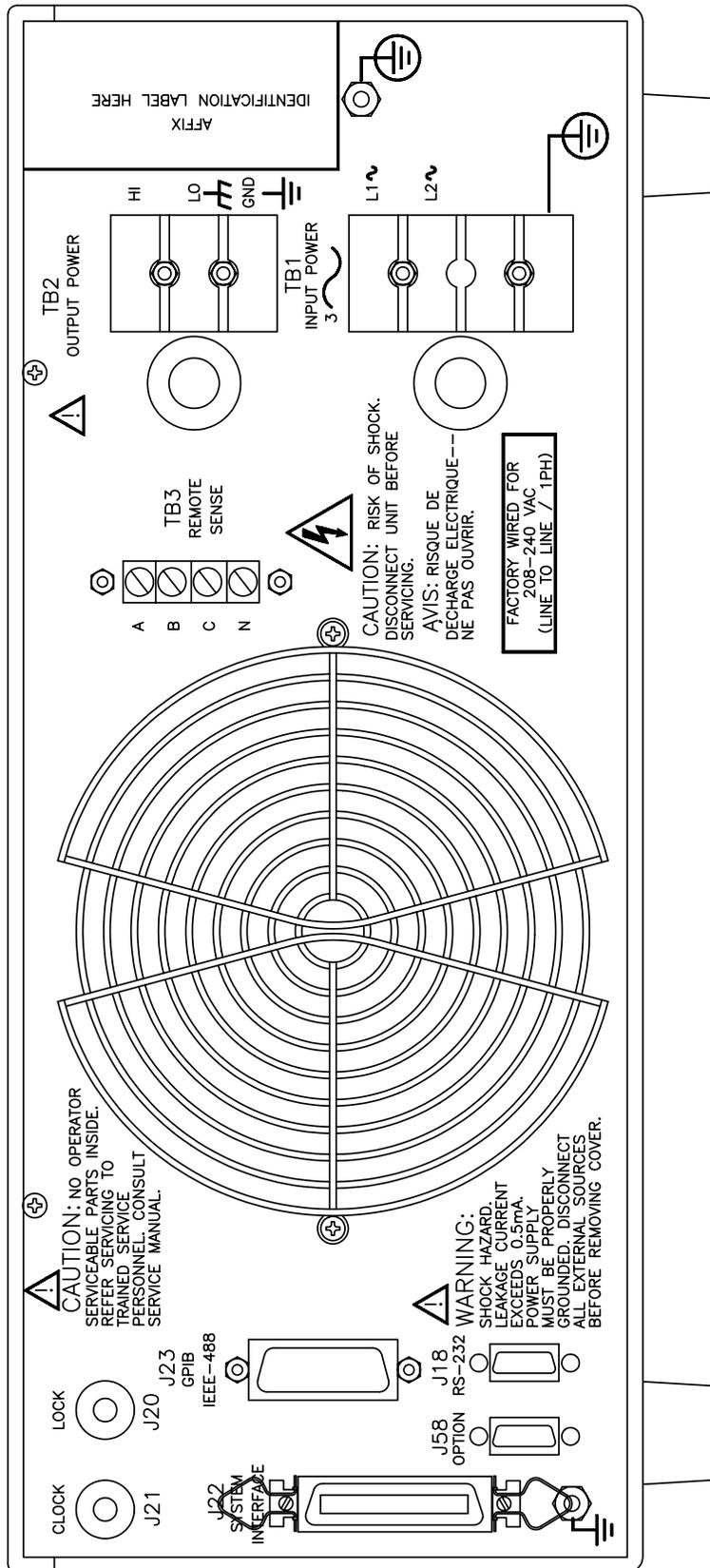
Figure 3-6: Rear Panel View for the 5001i/5001iX
