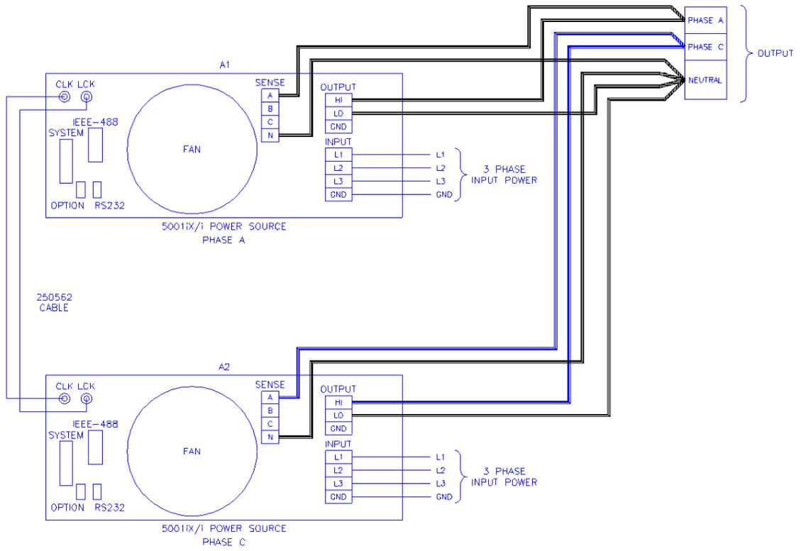
Figure 3-15: Three-Phase 9000 VA System (9003iX/i – One Controller)
