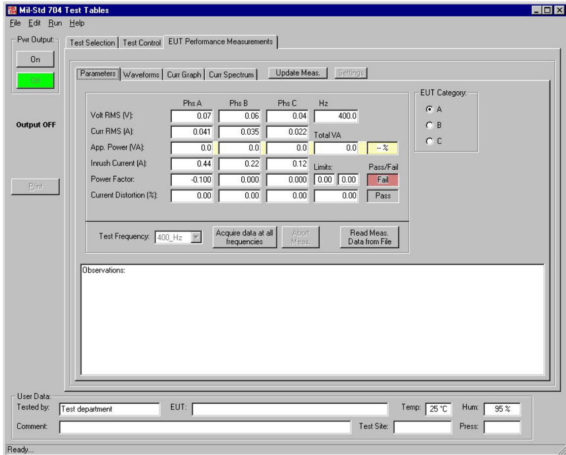
Figure 9-65: 704 Option EUT Measurement Data Screen.
