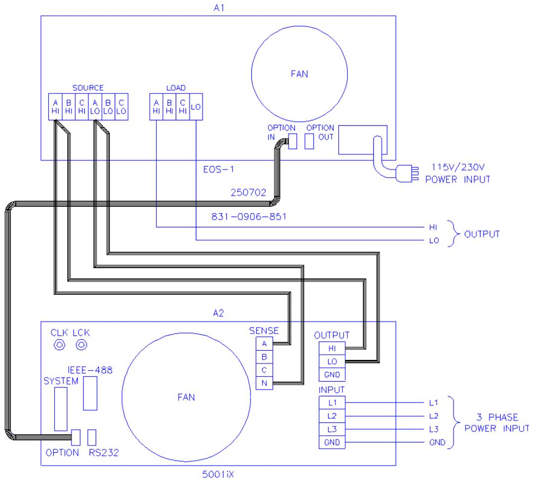
Figure 9-37: Example Connection With Compliance Test System and EOS-1
