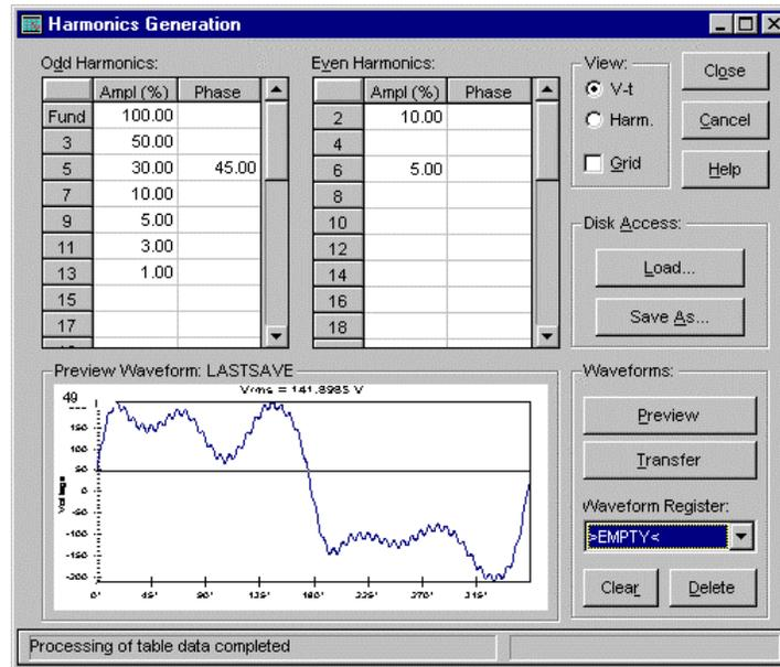
Figure 4-30: Custom waveform creation with GUI program
