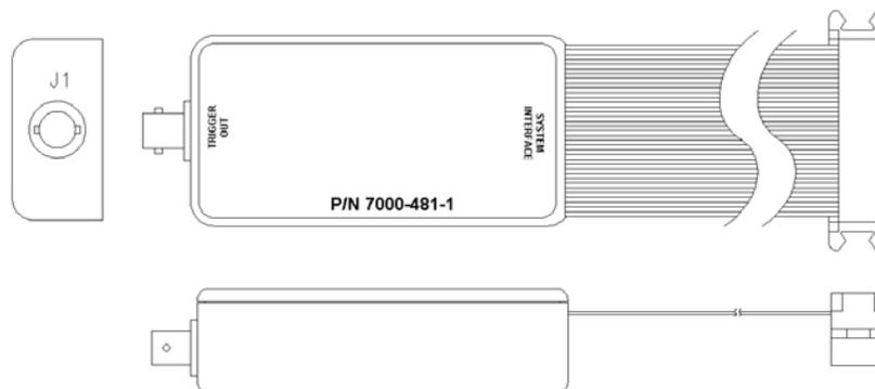
Figure 3-4: Function Strobe / Trigger Output Accessory.
