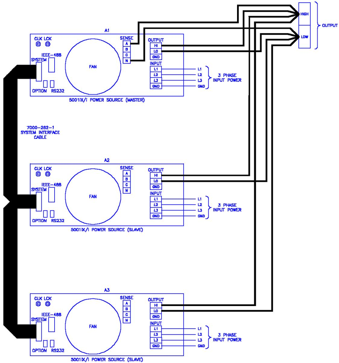
Figure 3-12: Three-Phase 15000 VA system (15003iX/i - One Controller)
