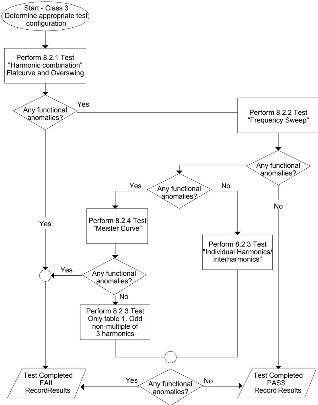
Figure 9-33: IEC 61000-4-13 Test Flowchart Class 3
