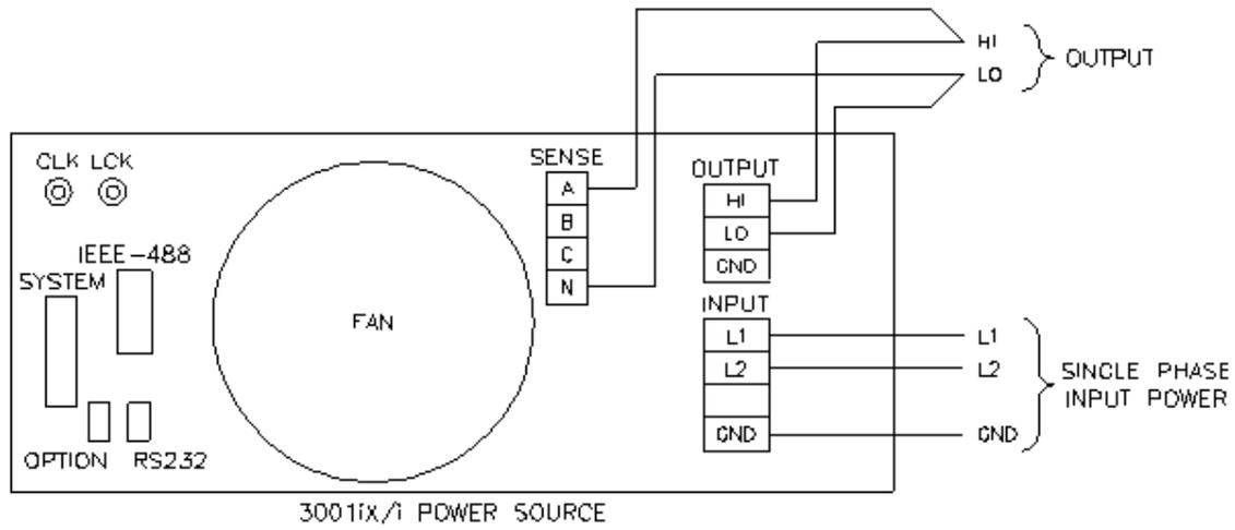
Figure 3-8: Functional Test Setup
