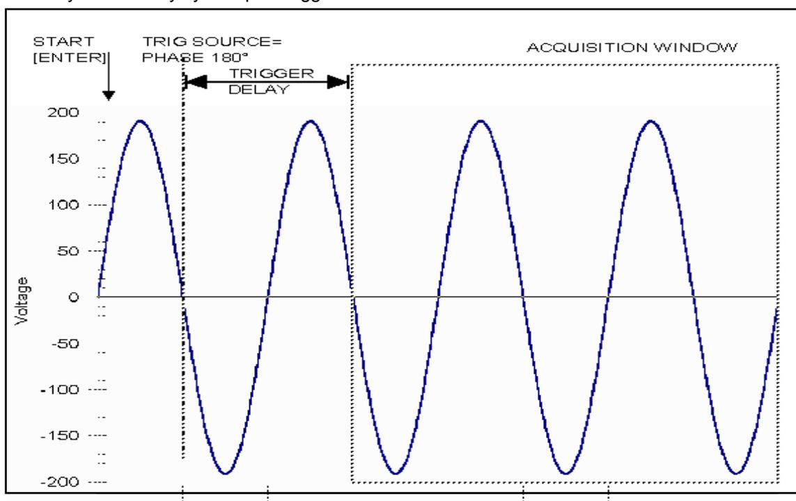
Figure 4-37: Positive trigger delay (Post trigger data)
