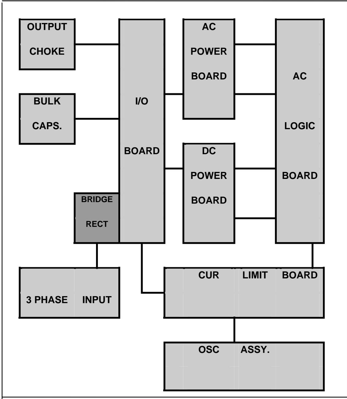
Figure 5-1: AC Power System Block Diagram
