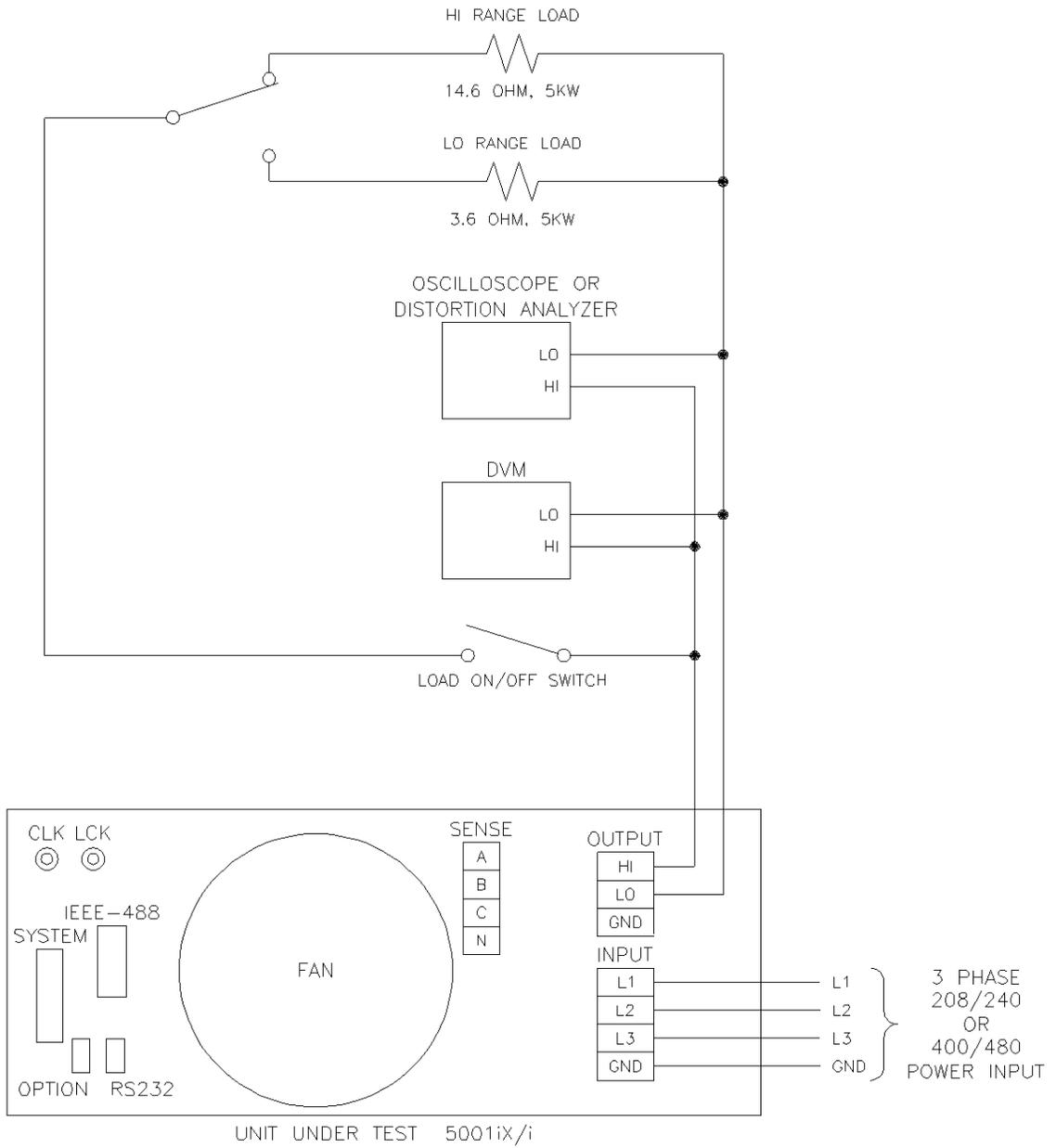
Figure 3-9: Single Phase 10000 VA System (1000iX/i)
