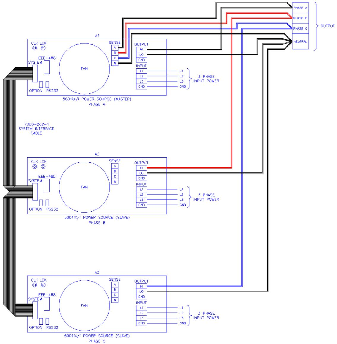
Figure 3-13: Connection With MODE Option
