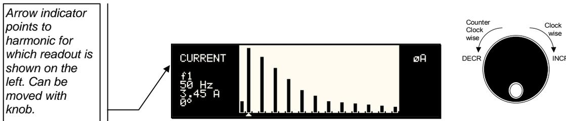
Figure 4-34: Scrolling through bar chart FFT data
