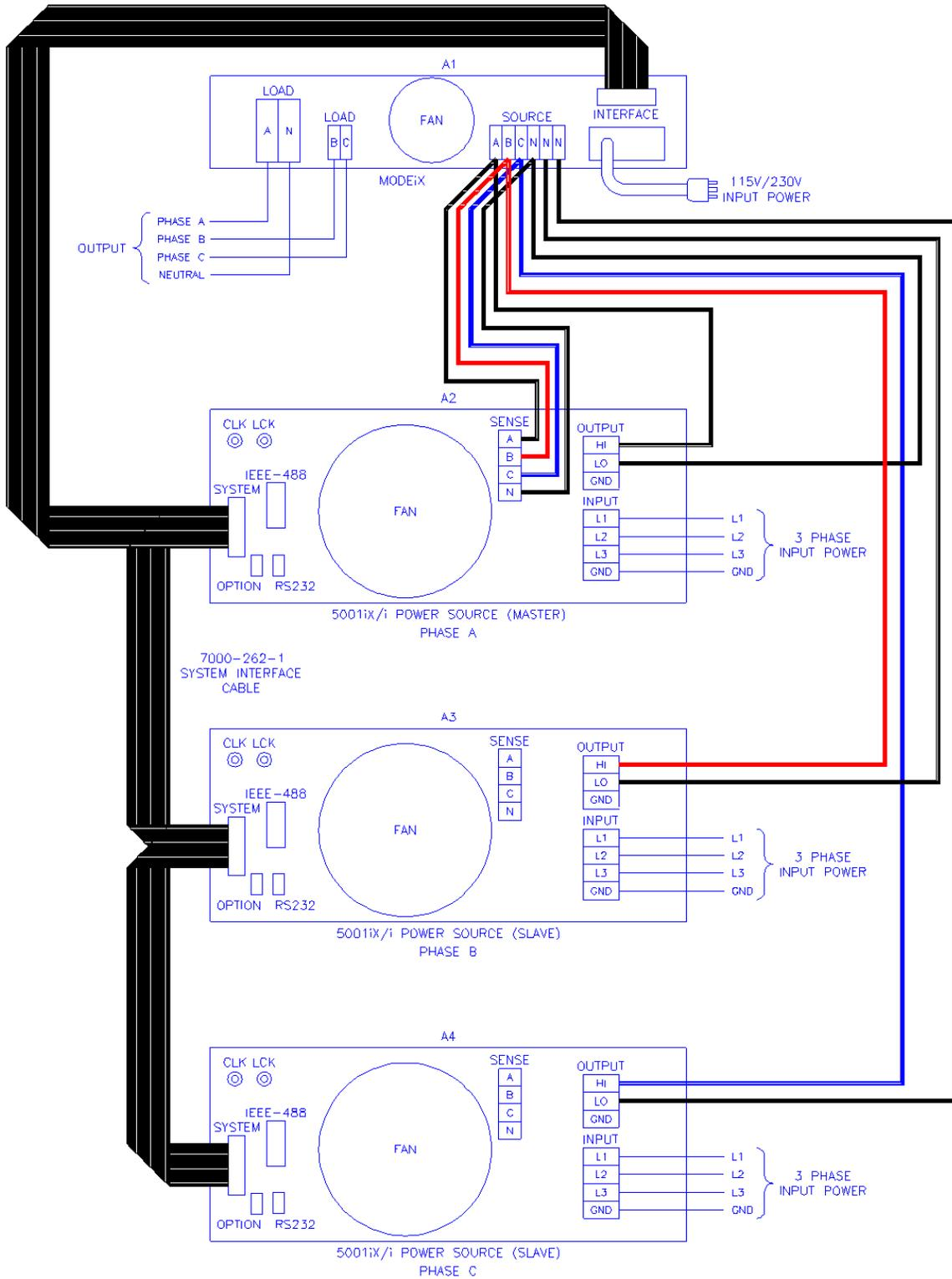
Figure 3-14: Two Phase 10000 VA System (10002i-LK Two Controllers)
