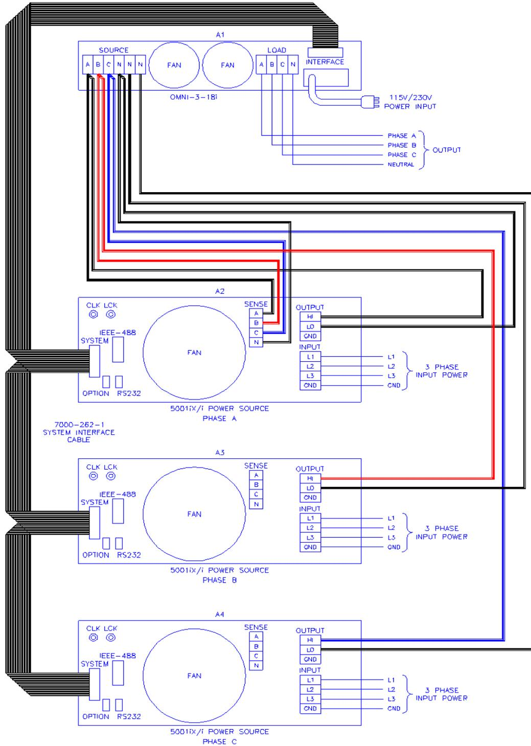
Figure 9-44: Schematic Showing OMNI 1-37i and 1-37j Connected to 5001iX System
