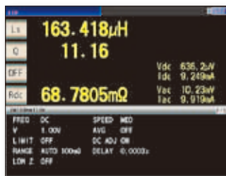
L/Q Rdc continuous measurement screen L/Q (1 kHz, 1 mA constant current measurement) and Rdc (DC measurement) display screen
