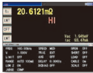
LCR mode Rs display screen (100 kHz measurement)
