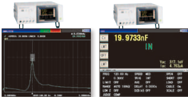
Frequency sweep measurement Z peak comparator screen
