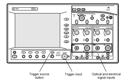
Figure 2-3. Trigger Controls
