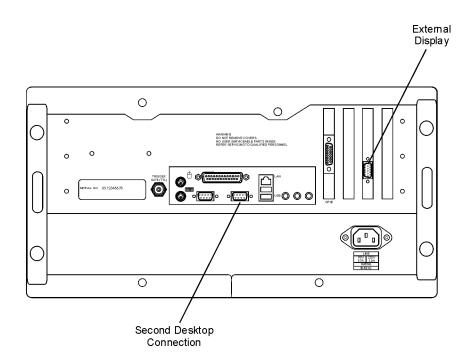
Figure 1-26. External Monitor Connector
