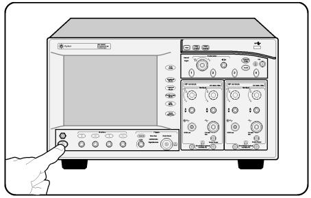
Figure 1-6. ON/OFF Switch
