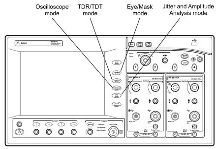
Figure 2-1. The Four Instrument Modes
