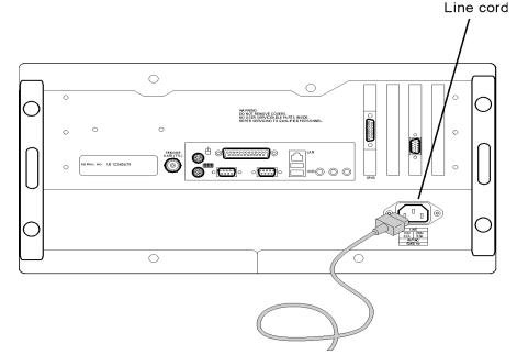
Figure 1-5. Line Cord Connector on 86100C Rear Panel
