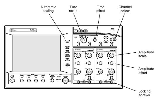
Figure 2-6. Amplitude and time adjustments
