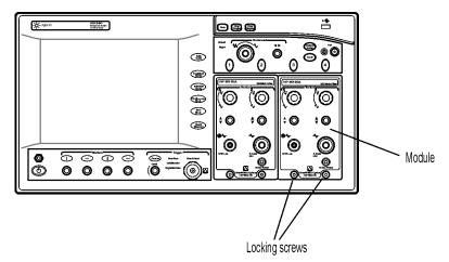
Figure 1-2. Installing a Module
