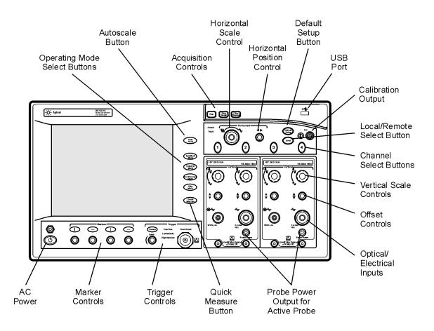
Figure 2-4. Front-Panel Features
