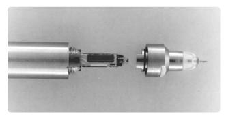
A replaceable state-of-the-art GaAs IC provides high performance and extends the lifetime of the 85024A.
