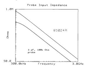
Probe with less error due to higher input impedance. For example, in a 50 ohm system at 500 MHz, the 85024A presents 455 ohms which produces a 10% signal loss from loading effects, while a 3 pF, 100 k $\Omega$  probe presents 106 ohms causing a 32% signal loss.
