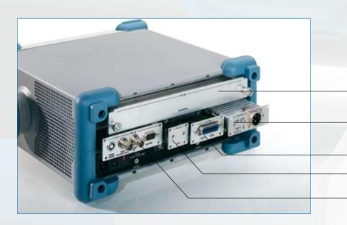
\_\_\_\_ Battery pack (R&S®FSL-B31)
