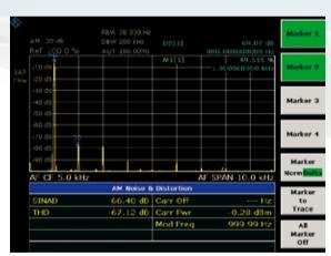
THD measurement on an amplitude-modulated signal The first harmonic of the modulation signal is well suppressed by 69 dB. This corresponds to a THD (D2) of less than 0.1 %.
