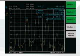
**Phase noise measurement with phase noise marker** The phase noise marker provides a quick measurement of the phase noise at a specific carrier offset. The result in dBc (1 Hz) includes all necessary corrections for the noise bandwidth of the filter, the detector used, and averaging. The phase noise of typ. –103 dBc (1 Hz) at 10 kHz from the carrier is sufficient for a number of oscillator measuring tasks.
