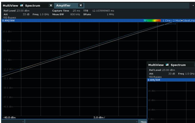
Gain transfer curve measurement (AM/AM) of an amplifier. For the curve above, a CW signal with a linear power ramp has been used as the stimulus. As expected, the AM/AM curve is a line. The curve on the right was measured using a digitally modulated signal generated by the R&S®FSW. The AM/AM is a cloud-like curve; the line width is due to amplifier memory effects.
