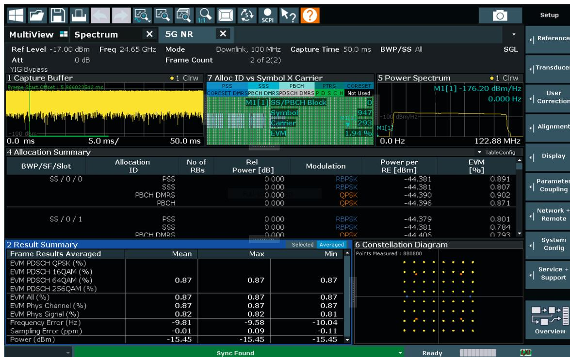
The R&S®FSW-K145 supports both the OFDMA and the transform precoded modes in the uplink.
