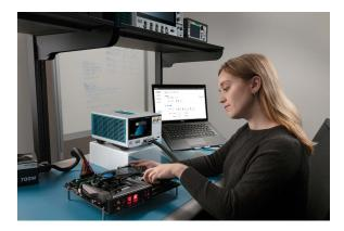
The TMT4 can be set up and ready to test in as little as 5 minutes, and an optimized user interface makes testing easier than ever. With this, Tektronix has responded to the needs of the modern engineer when it comes to the evaluation of link health in PCIe Gen 3 and Gen 4 devices.
