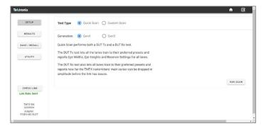
To access the web-based browser interface, the user must connect the Margin Tester via the Ethernet port located on the back of the instrument to either a local network or point-to-point to a PC. The Margin Tester has a dedicated IP address that is configured once connected to a local network or PC, allowing the user to connect to the UI by inputting the IP address shown on the Margin Tester into a supported web browser, which includes Google Chrome, Firefox, and Microsoft Edge.
