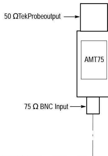
Figure 2: Connecting the AMT75 adapter
